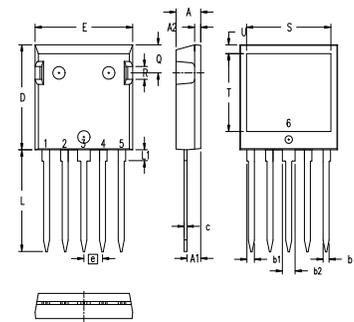
NOTE: Bottom heatsink meets 3000 Volts AC 1 sec isolation to the other pins.
