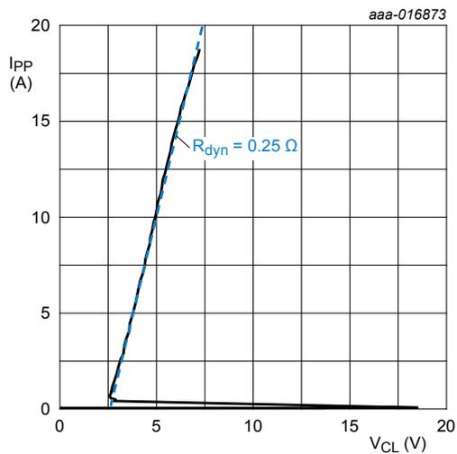
$t_p = 100 \text{ ns}$ ; Transmission Line Pulse (TLP)
