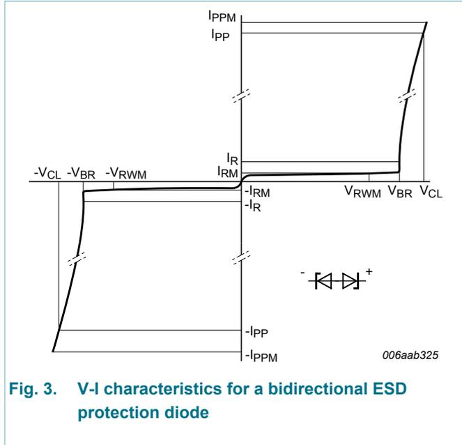
Fig. 3. V-I characteristics for a bidirectional ESD protection diode
