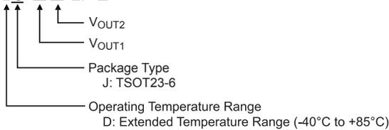
\*\* For RoHS Compliant Packaging, add suffix - LF (e.g. MP2004DJ-□□-LF); For Tape and Reel, add suffix -Z (e.g. MP2004DJ-□□-LF-Z).
