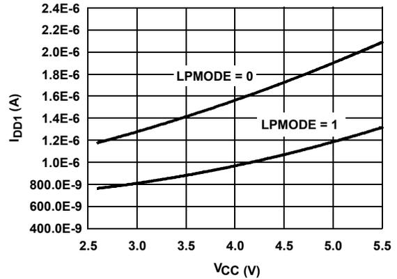
FIGURE 4. I<sub>DD1</sub> vs V<sub>CC</sub> WITH LPMODE ON AND OFF
