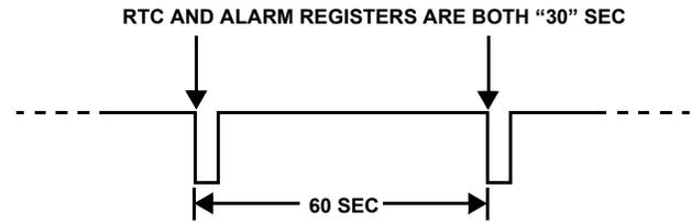
Note that the status register ALM bit will be set each time the alarm is triggered, but does not need to be read or cleared.
