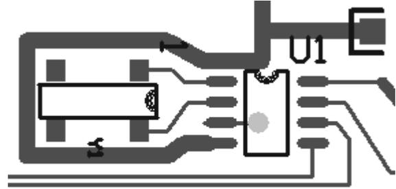
FIGURE 19. SUGGESTED LAYOUT FOR ISL1220 AND CRYSTAL
