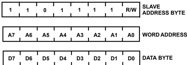
FIGURE 15. SLAVE ADDRESS, WORD ADDRESS, AND DATA BYTES
