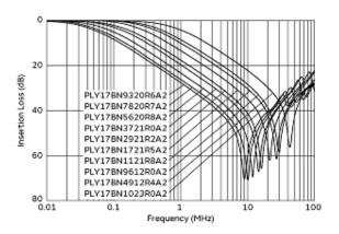
Common Mode Insertion Loss-Frequency Characteristics
