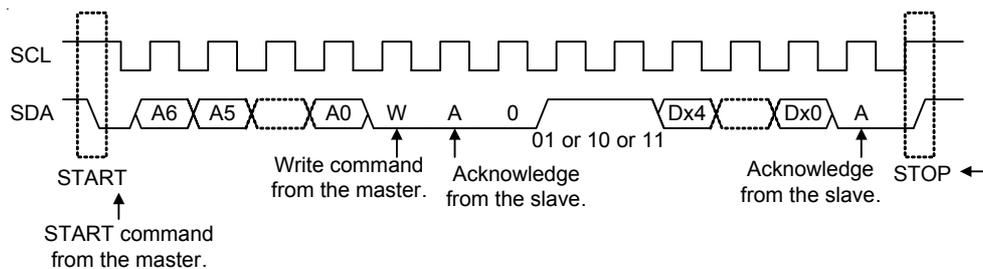
Figure 1. I<sup>2</sup>C Transmission Flow in the RT9941
