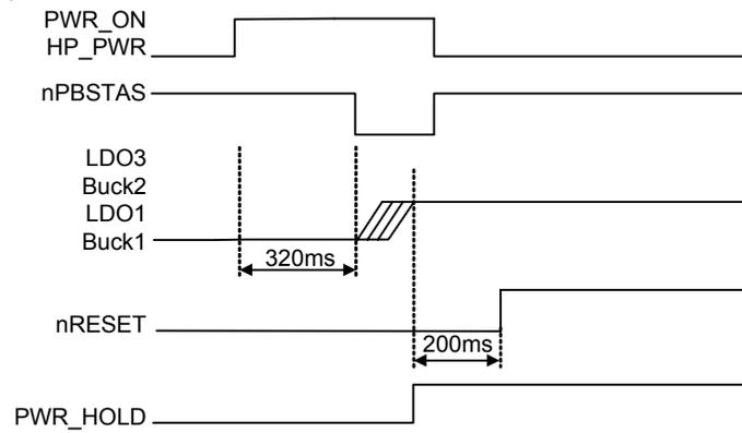
Figure 11. PWR\_ON & HP\_PWR & nPBSTAS Timing Diagram
