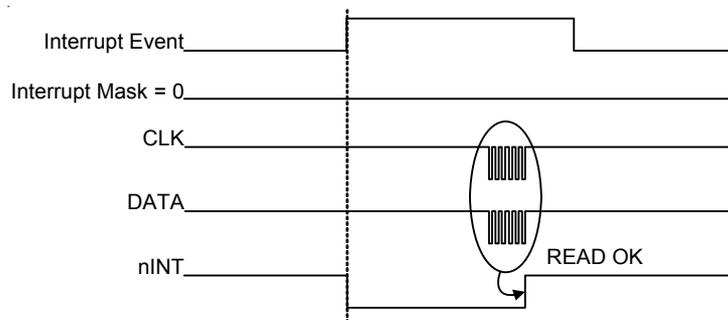
Figure 9. Interrupt without Mask
