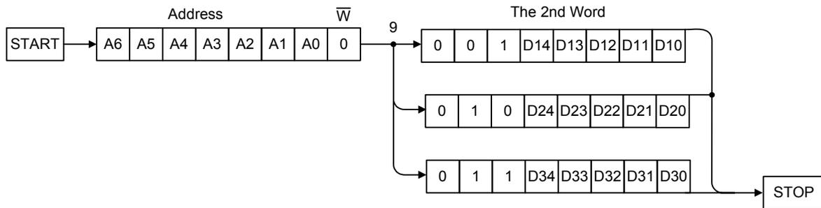
Figure 3. I<sup>2</sup>C One Command Flow in the RT9941
