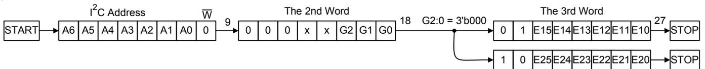
Figure 4. I<sup>2</sup>C Two Commands Flow in the RT9941
