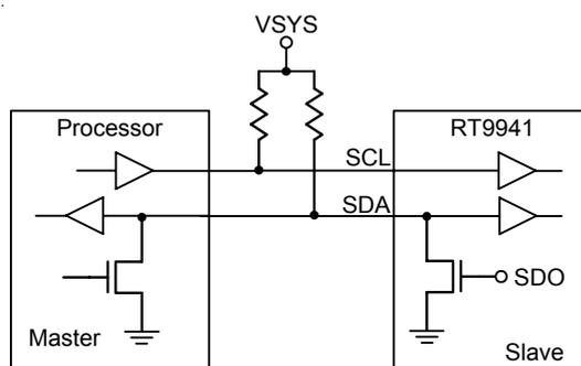
Figure 2. I<sup>2</sup>C Function Block in the RT9941
