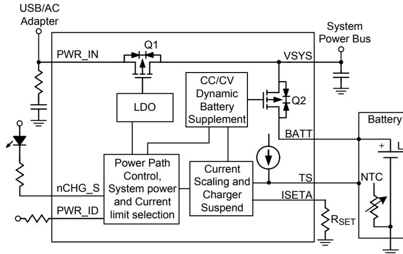
Figure 13. Charger Block Diagram and Required External Components
