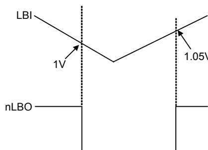
Figure 23. Typical LBI Rising and Falling Threshold Voltage.
