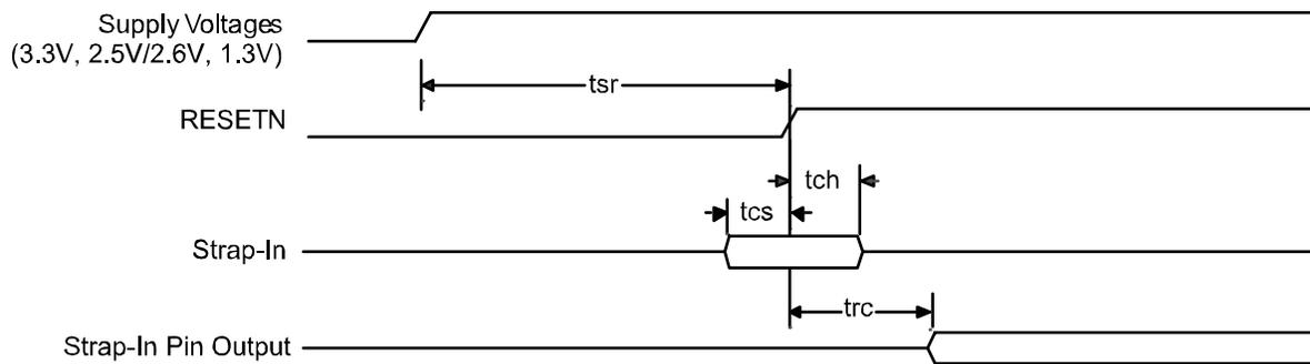
Figure 16. Reset Timing
