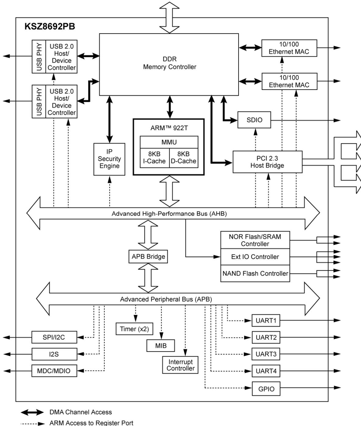
Figure 3. KSZ8692PB, KSZ8692PB-S Functional Block Diagram
