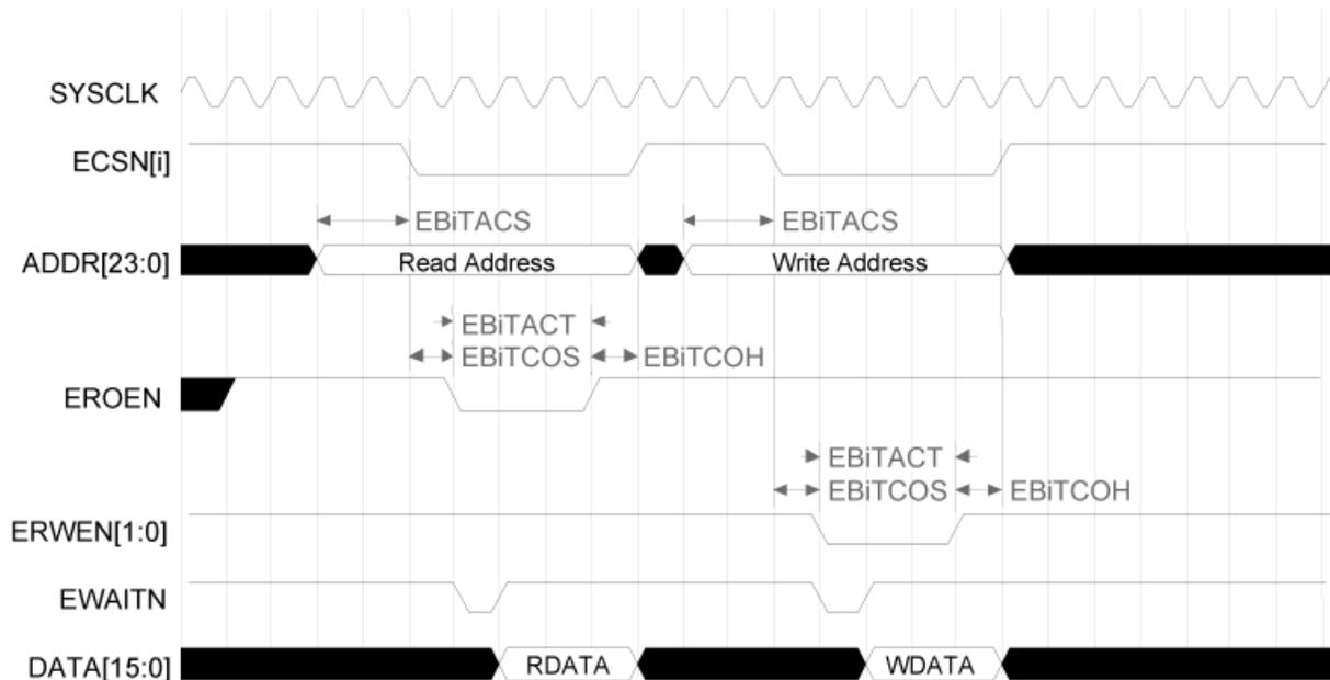
Figure 19. External I/O Read and Write Cycles
