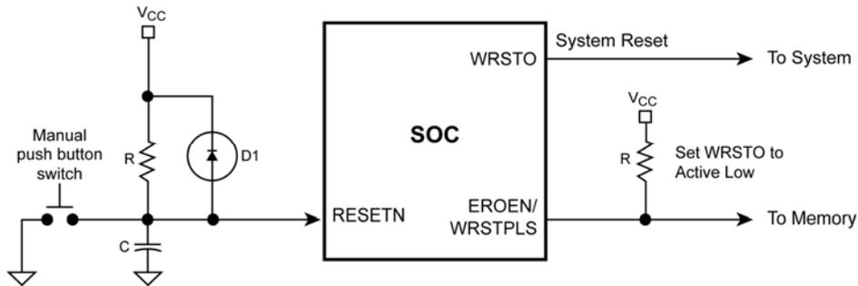
Figure 14. Reset Circuit
