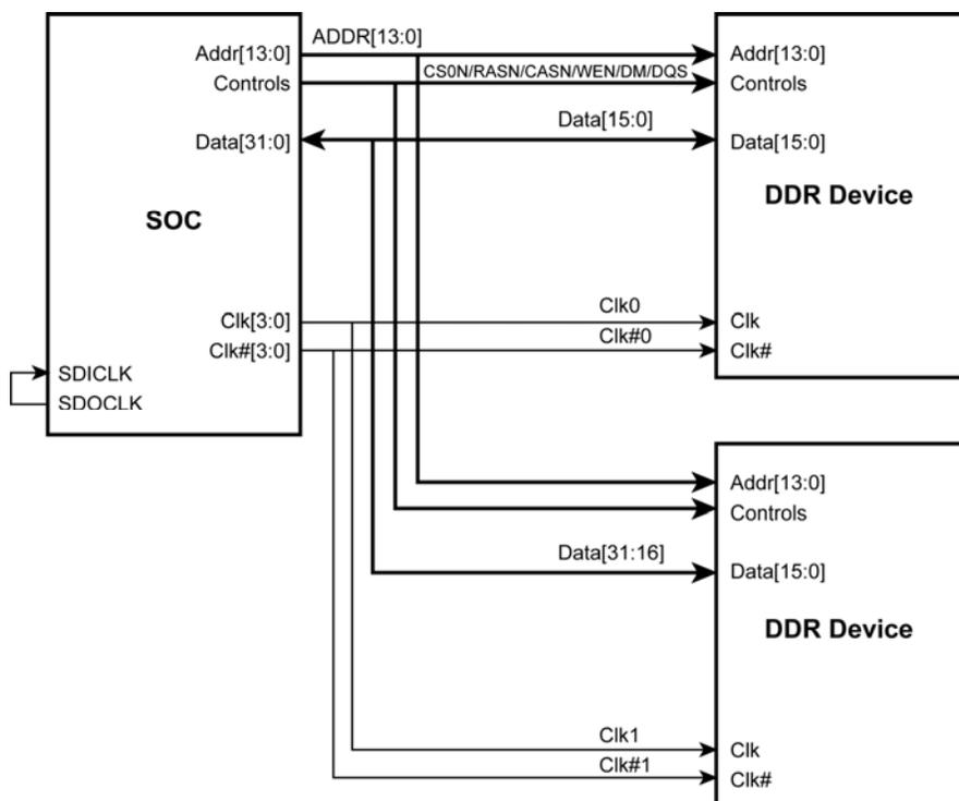
Figure 8. Single 16-bit DDR Memory Devices Interface Example
