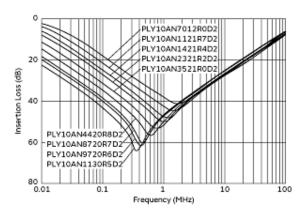
Common Mode Insertion Loss (Typ.)
