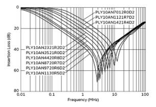
Differential Mode Insertion Loss (Typ.)
