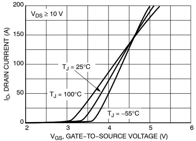
Figure 2. Transfer Characteristics
