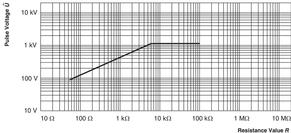
Pulse load rating in accordance with IEC 60115-1, 4.27; 10  $\mu$ s/700  $\mu$ s;
