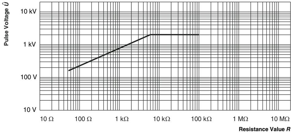
Pulse load rating in accordance with IEC 60115-1, 4.27; 1.2  $\mu$ s/50  $\mu$ s;
