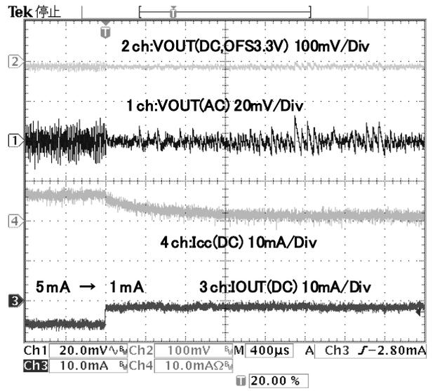
Figure 23. I<sub>o</sub> change 5mA=>1mA, VIN=2.8V[CR2032]
