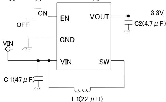
Figure 1. Application Circuit
