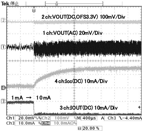
Figure 24. I<sub>o</sub> change 1mA=>10mA, VIN=2.8V[CR2032]
