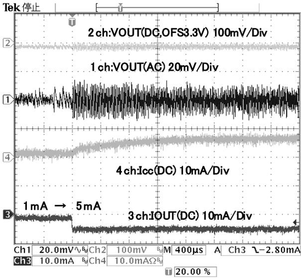
Figure 22. I<sub>o</sub> change 1mA=>5mA, VIN=2.8V[CR2032]
