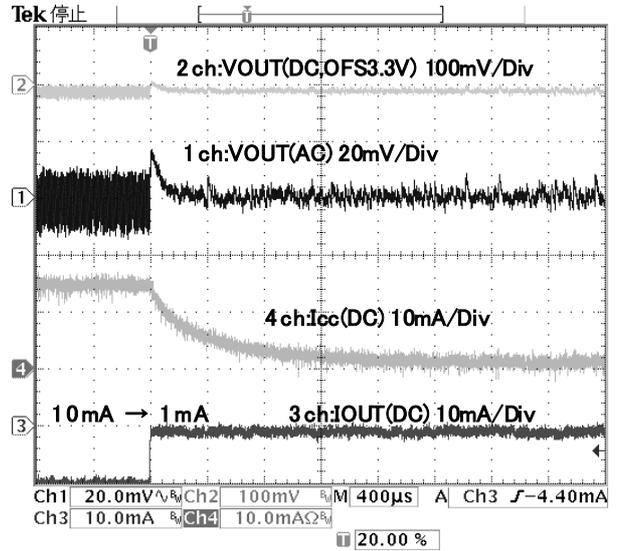
Figure 25. I<sub>o</sub> change 10mA=>1mA, VIN=2.8V[CR2032]
