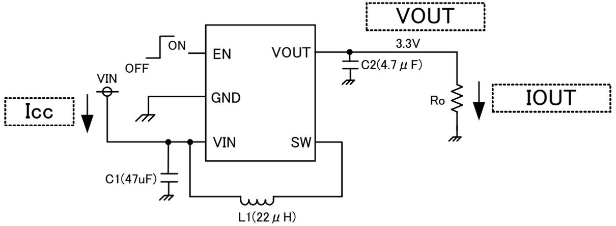
Figure 17. Measure circuit
