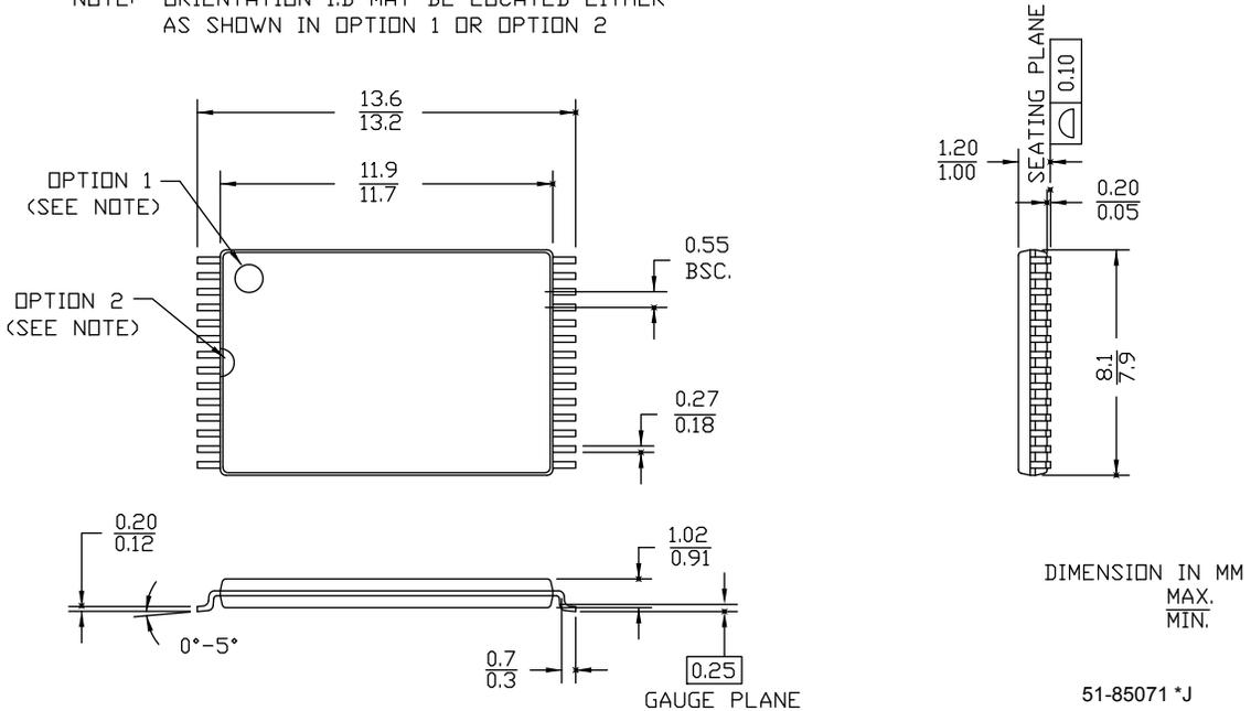
Figure 13. 28-pin TSOP I (8 × 13.4 mm) Package Outline - Reverse, 51-85074
