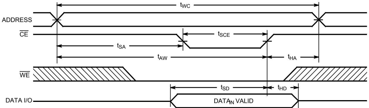
Figure 9. Write Cycle No. 3 ( $\overline{WE}$  Controlled,  $\overline{OE}$  LOW) [18, 20]
