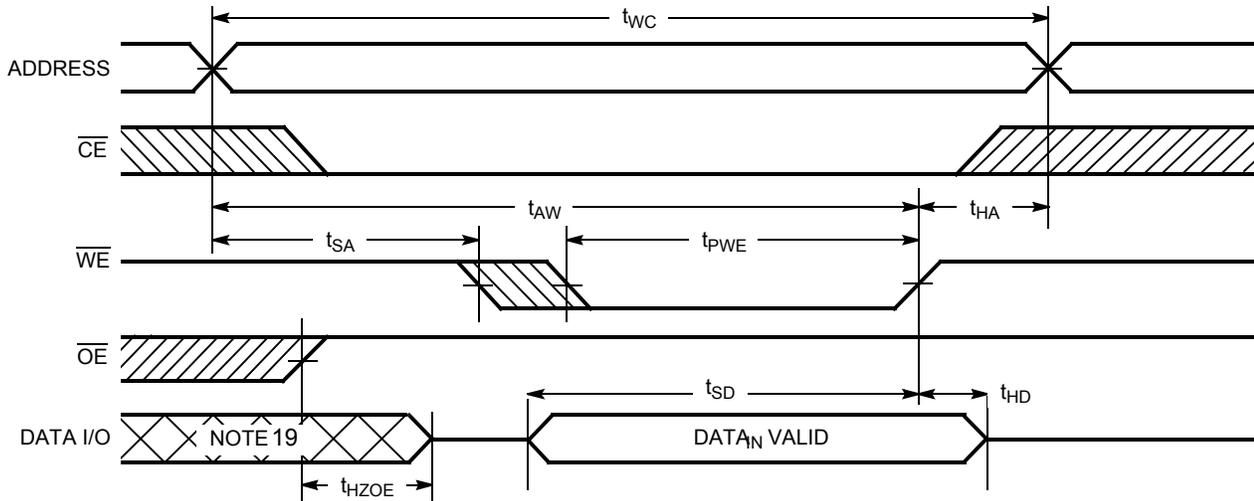
Figure 8. Write Cycle No. 2 ( $\overline{CE}$  Controlled) [16, 17, 18]
