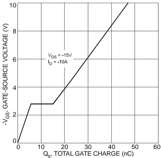
Fig. 14 Gate-Charge Characteristics
