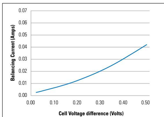
**Figure 2.** Balancing current versus cell voltage differential.
