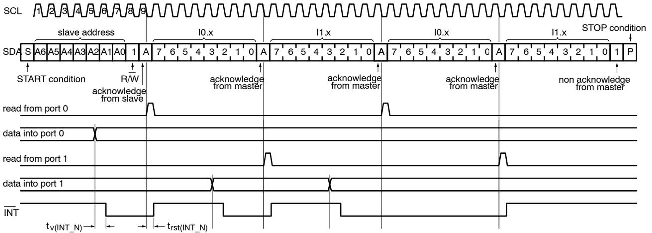
**Figure 9. Read from Input Port Register, Scenario 1**
