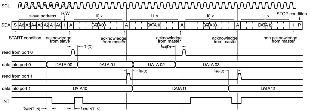
**Figure 10. Read from Input Port Register, Scenario 2**
