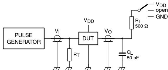
$R_L$  = load resistor.
