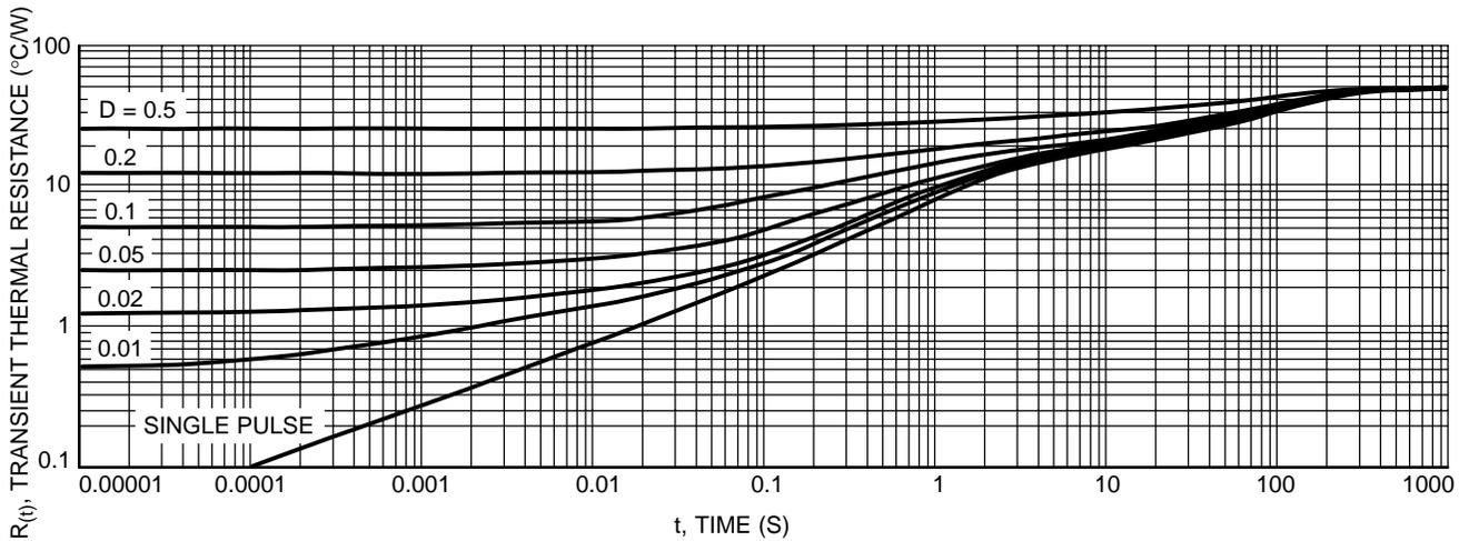
Figure 8. Thermal Response, Junction-to-Ambient (1 inch pad)
