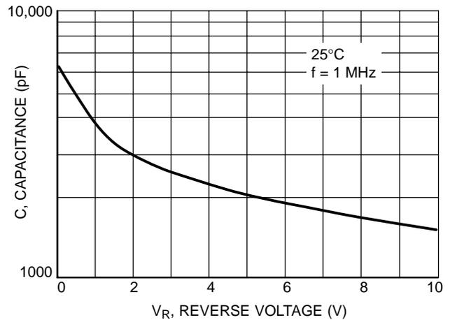
Figure 4. Typical Capacitance
