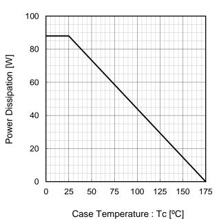
Fig.7 Ip-Tc Derating Curve
