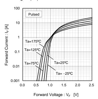
Fig.2 V<sub>F</sub> - I<sub>F</sub> Characteristics
