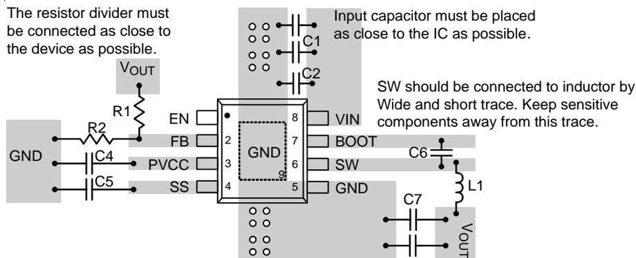
(c). For SOP-8 (Exposed) Package
