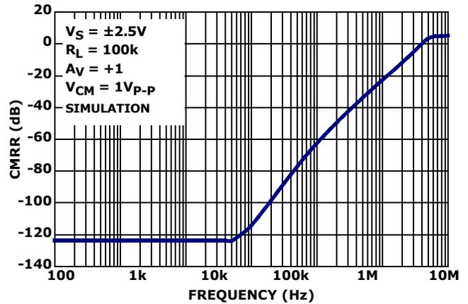
FIGURE 22. CMRR vs FREQUENCY,  $V_S = \pm 2.5V$
