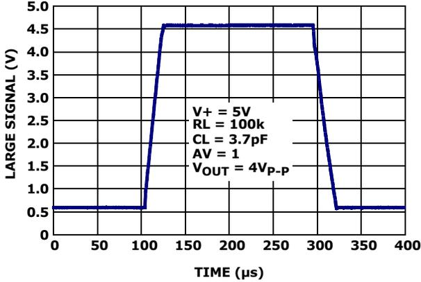
FIGURE 53. CHARACTERIZED LARGE SIGNAL STEP RESPONSE (4V)
