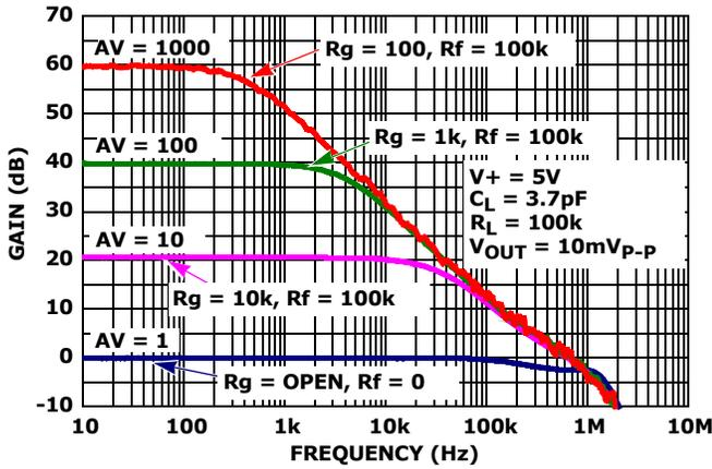
FIGURE 19. FREQUENCY RESPONSE vs CLOSED LOOP GAIN
