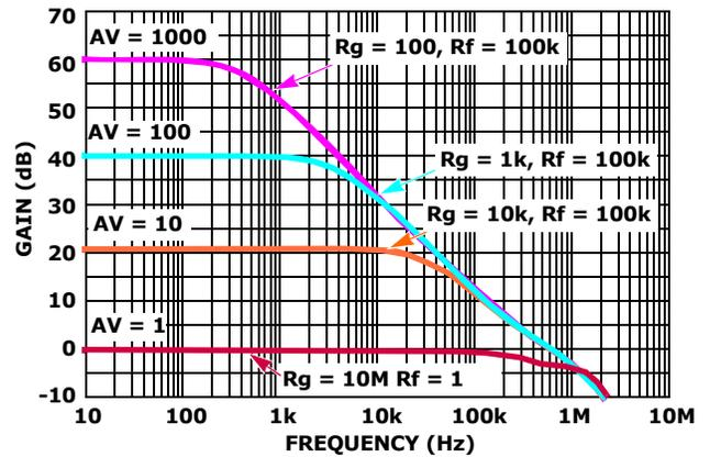
FIGURE 50. SIMULATED FREQUENCY RESPONSE vs CLOSED LOOP GAIN
