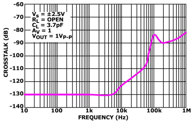
FIGURE 33. Crosstalk vs Frequency,  $V_S = \pm 2.5V$
