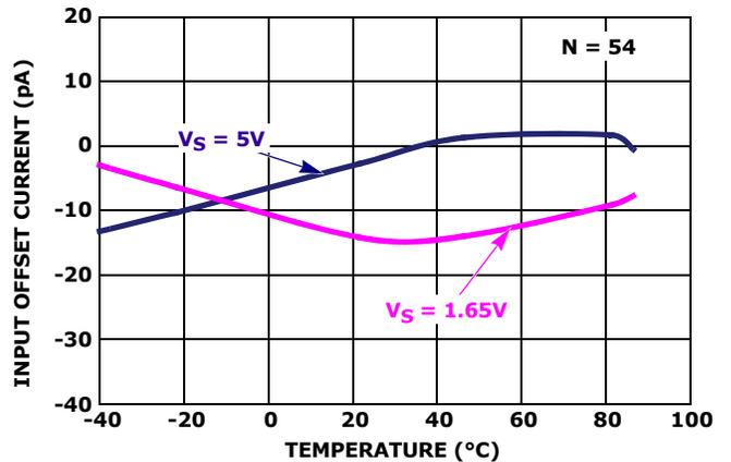
FIGURE 6. MEDIAN  $I_{OS}$  vs SUPPLY VOLTAGE vs TEMPERATURE
