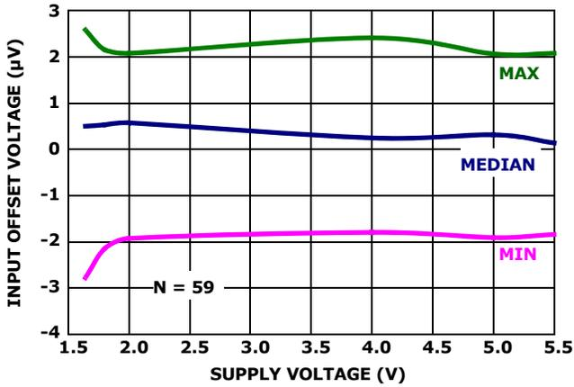
FIGURE 1. INPUT OFFSET VOLTAGE vs SUPPLY VOLTAGE
