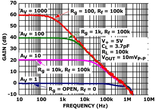
FIGURE 49. CHARACTERIZED FREQUENCY RESPONSE vs CLOSED LOOP GAIN
