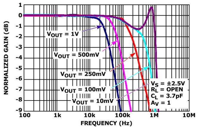
FIGURE 18. GAIN vs FREQUENCY vs  $V_{OUT}, R_L = \text{OPEN}$
