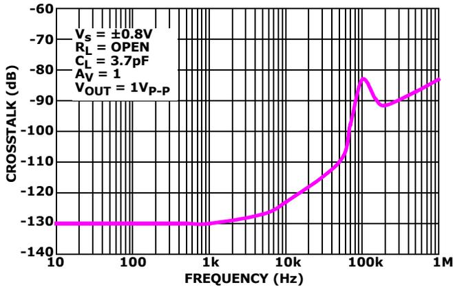
FIGURE 32. Crosstalk vs Frequency,  $V_S = \pm 0.8V$
