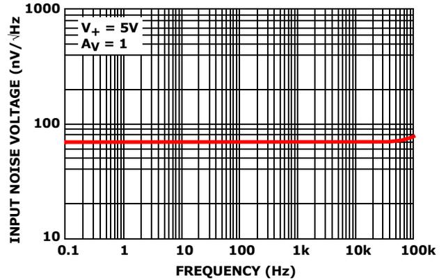
FIGURE 48. SIMULATED INPUT NOISE VOLTAGE DENSITY vs FREQUENCY
