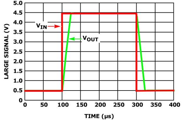
FIGURE 54. SIMULATED LARGE SIGNAL STEP RESPONSE (4V)
