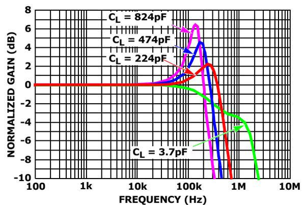
FIGURE 52. SIMULATED GAIN vs FREQUENCY vs  $C_L$
