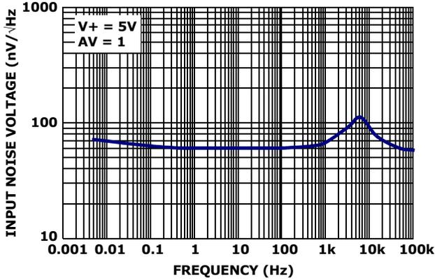
FIGURE 47. CHARACTERIZED INPUT NOISE VOLTAGE DENSITY vs FREQUENCY
