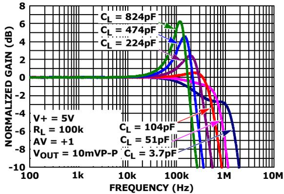
FIGURE 51. CHARACTERIZED GAIN vs FREQUENCY vs  $C_L$
