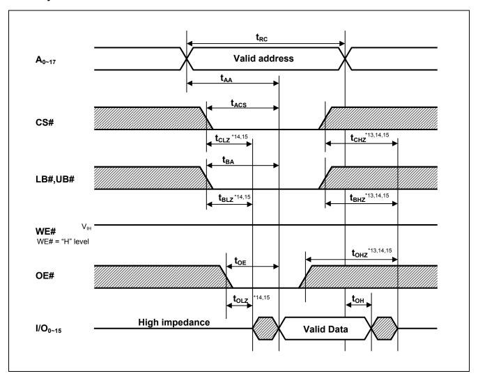
Note 13.  $t_{CHZ}$ ,  $t_{BHZ}$  and  $t_{OHZ}$  are defined as the time when the I/O pins enter a high-impedance state and are not referred to the I/O levels.
