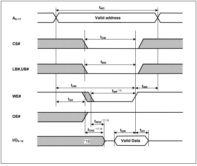
Note 16. t<sub>WP</sub> is the interval between write start and write end.
