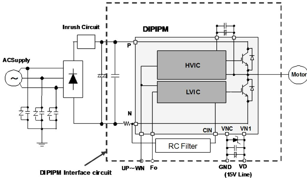
Fig.5-1-1 Demo board interface circuit
