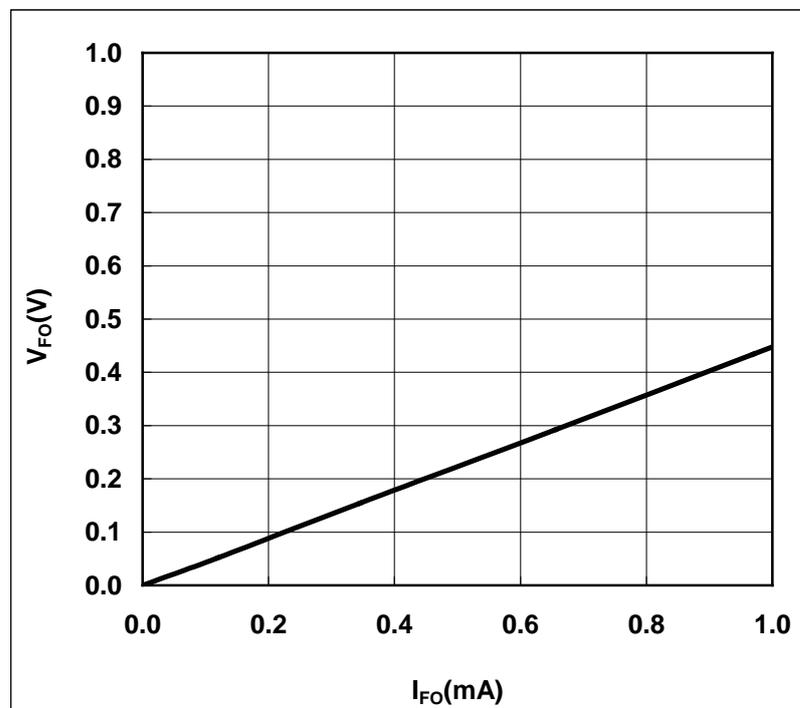
Fig.3-1-7 F<sub>o</sub> terminal typical V-I characteristics (V<sub>D</sub>=15V, T<sub>J</sub>=25°C)
