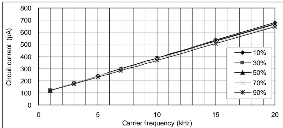
Fig.4-2-2  $I_{DB}$  vs. Carrier frequency for PSS10S92\*6-AG
