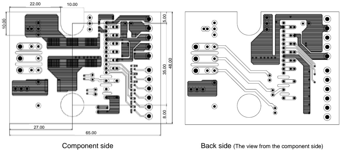
Fig.5-2-2 Demo board PCB pattern layout
