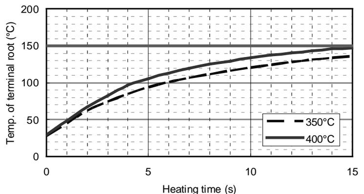
Fig.2-4-4 Temperature alteration of the terminal root (Example)
