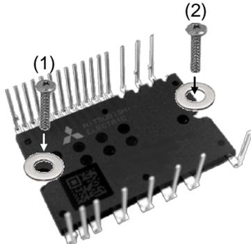
Fig.2-4-1 Recommended screw fastening order
