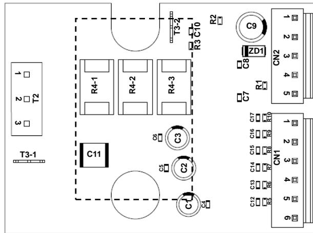
Fig.5-2-1 Demo board component layout (DIIPM is mounted to back side.)
