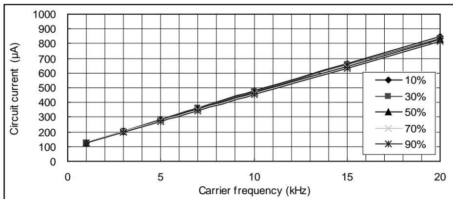
Fig.4-2-3  $I_{DB}$  vs. Carrier frequency for PSS15S92\*6-AG
