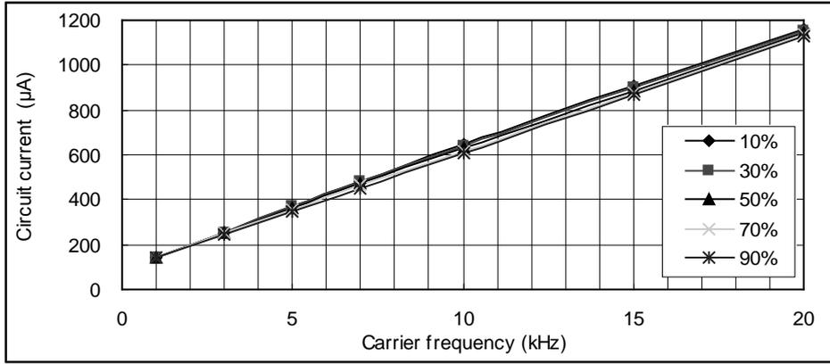
Fig.4-2-4  $I_{DB}$  vs. Carrier frequency for PSS20S92\*6-AG
