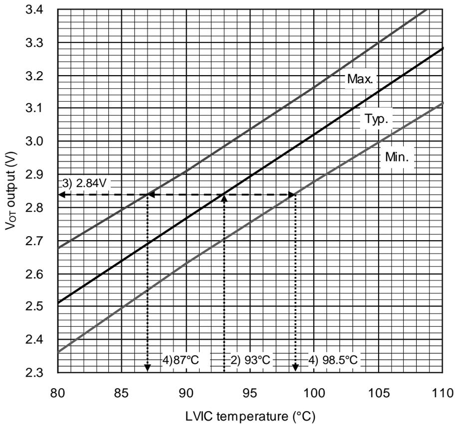
Fig.2-2-17 V<sub>OT</sub> output vs. LVIC temperature (Enlarged graph of Fig.2-2-14)
