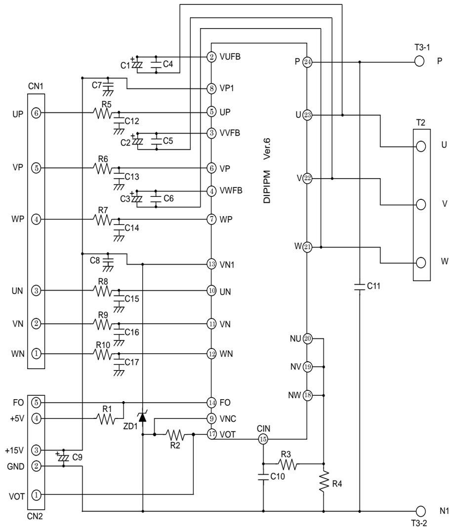
Fig.5-3-1 Demo board circuit schematic
