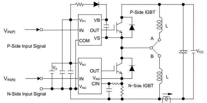
Fig.2-1-5 Evaluation circuit (inductive load)
