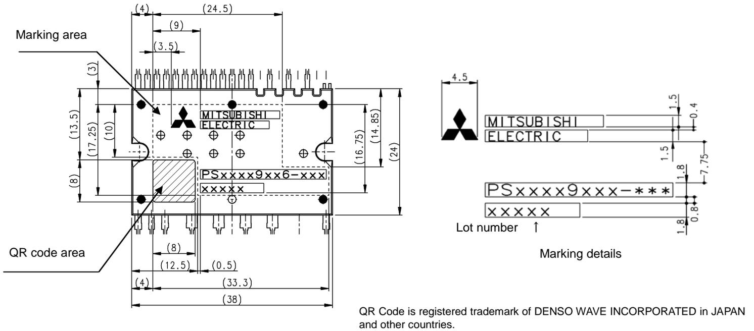
Fig.2-3-2 Laser marking view
