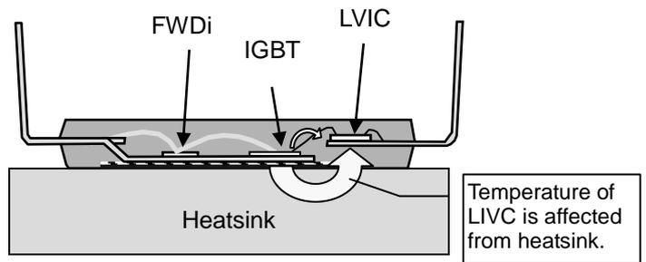
Fig.2-2-9 Thermal conducting from power chips
