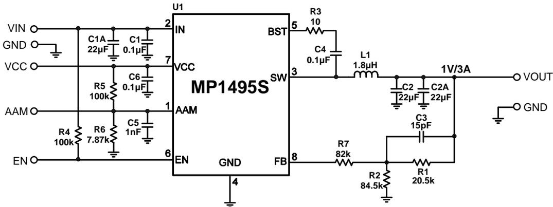
**Figure 12: 12V<sub>IN</sub>, 1V/3A Output**
