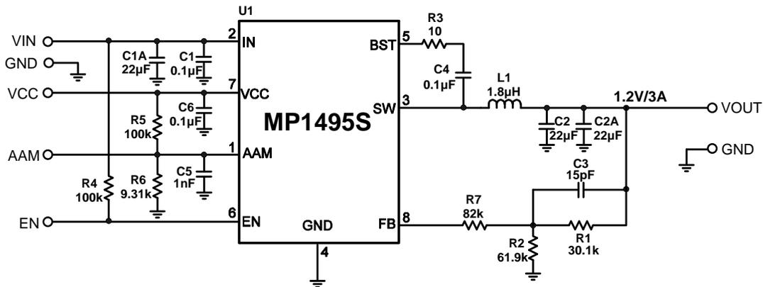
**Figure 11: 12V<sub>IN</sub>, 1.2V/3A Output**
