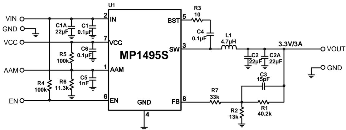
Figure 8: 12V<sub>IN</sub>, 3.3V/3A Output
