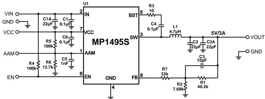
Figure 7: 12V<sub>IN</sub>, 5V/3A Output
