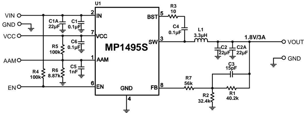
**Figure 10: 12V<sub>IN</sub>, 1.8V/3A Output**
