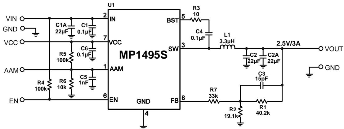
Figure 9: 12V<sub>IN</sub>, 2.5V/3A Output
