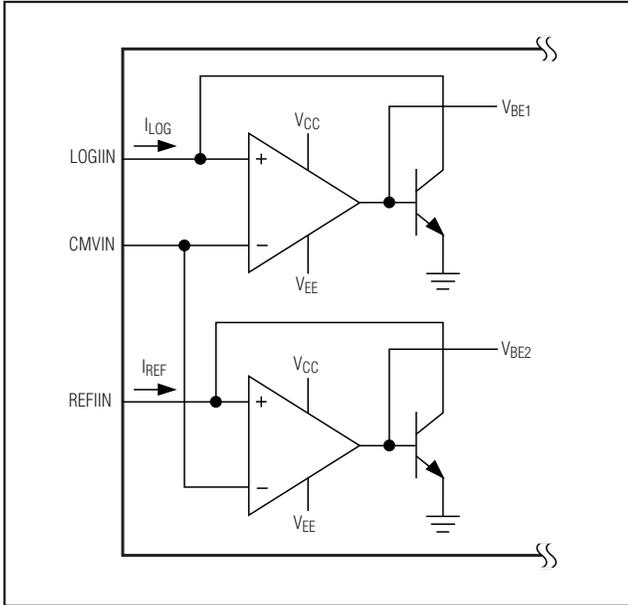
Figure 2. Simplified Model of a Logarithmic Amplifier
