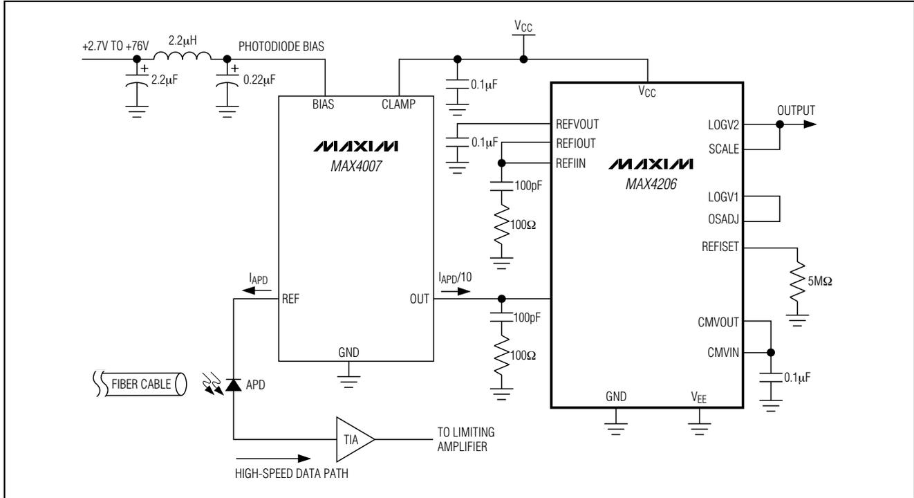
Figure 8. Logarithmic Current-Sensing Amplifier with Sourcing Input
