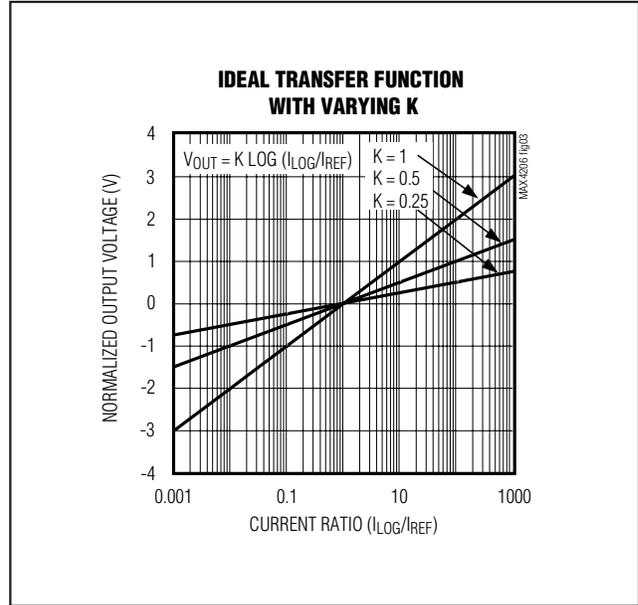
Figure 3. Ideal Transfer Function with Varying K
