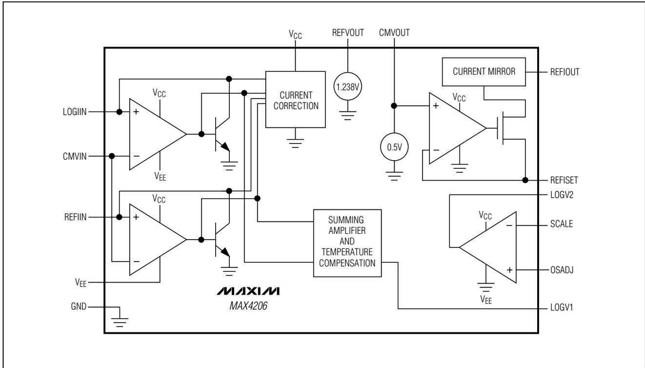
Figure 1. Functional Diagram
