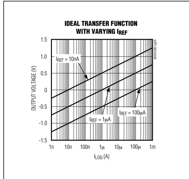
Figure 4. Ideal Transfer Function with Varying  $I_{REF}$
