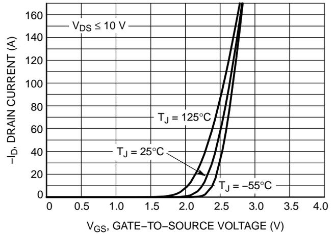
Figure 2. Transfer Characteristics
