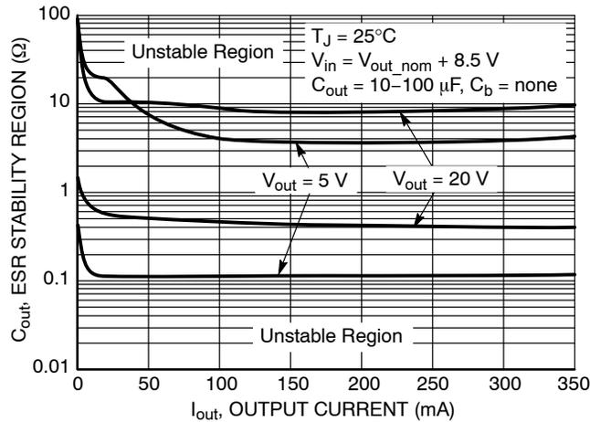
Figure 17.  $C_{out}$  ESR Stability Region vs. Output Current
