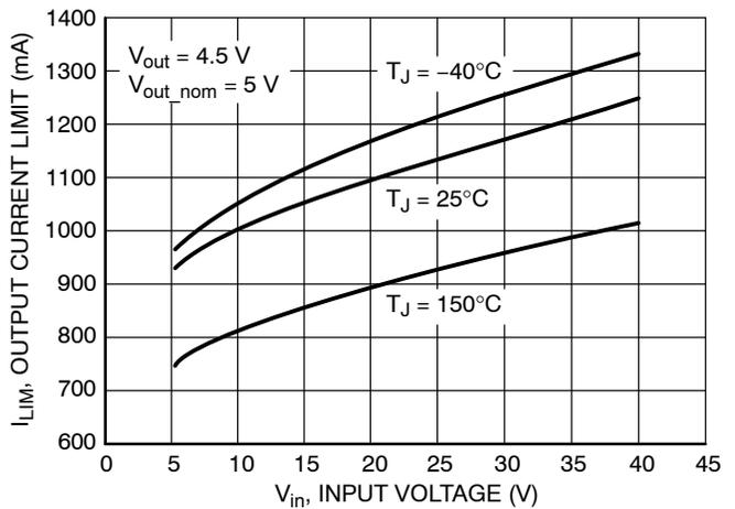
Figure 8. Output Current Limit vs. Input Voltage
