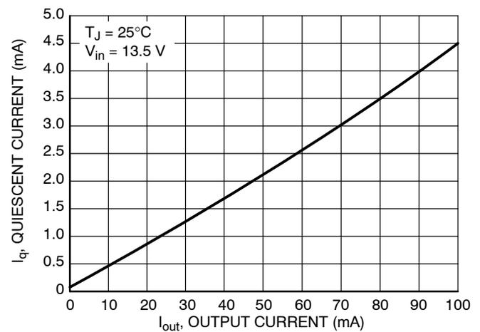
Figure 14. Quiescent Current vs. Output Current (Low Load)
