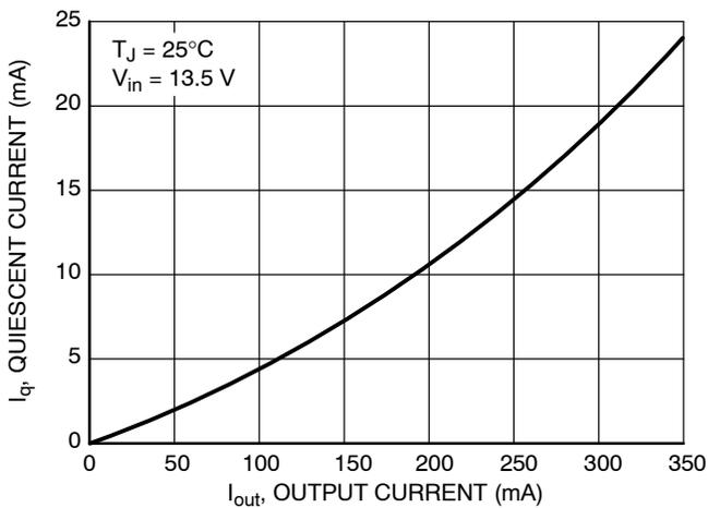
Figure 13. Quiescent Current vs. Output Current (High Load)
