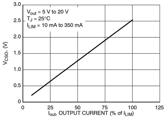
Figure 10. Output Current (% of  $I_{LIM}$ ) vs. CSO Voltage
