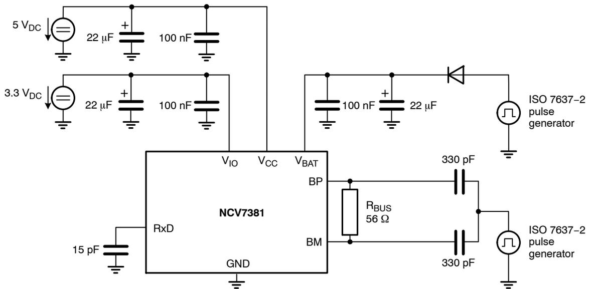
Figure 18. Test Setup for Measuring the Transient Immunity
