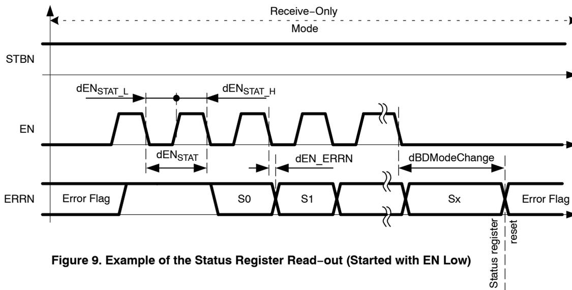
**Figure 9. Example of the Status Register Read-out (Started with EN Low)**
