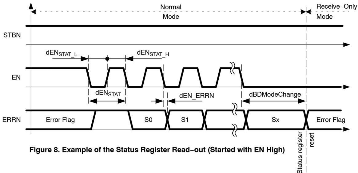
**Figure 8. Example of the Status Register Read-out (Started with EN High)**
