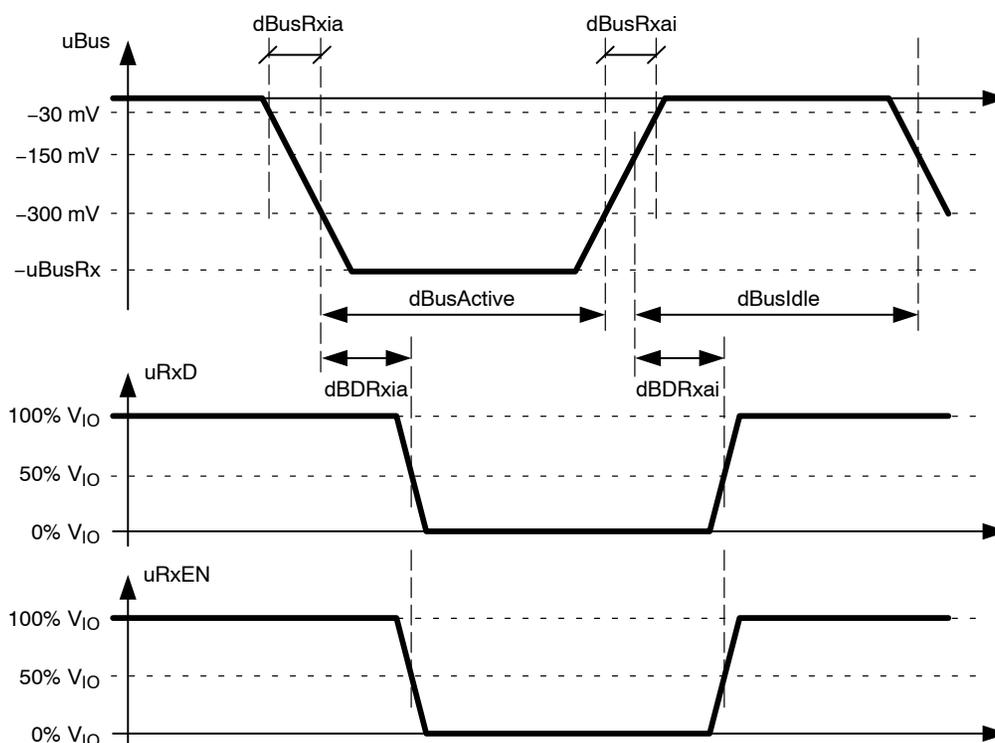
Figure 13. Parameters of Bus Activity Detection
