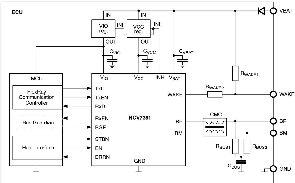
Figure 2. Application Diagram
