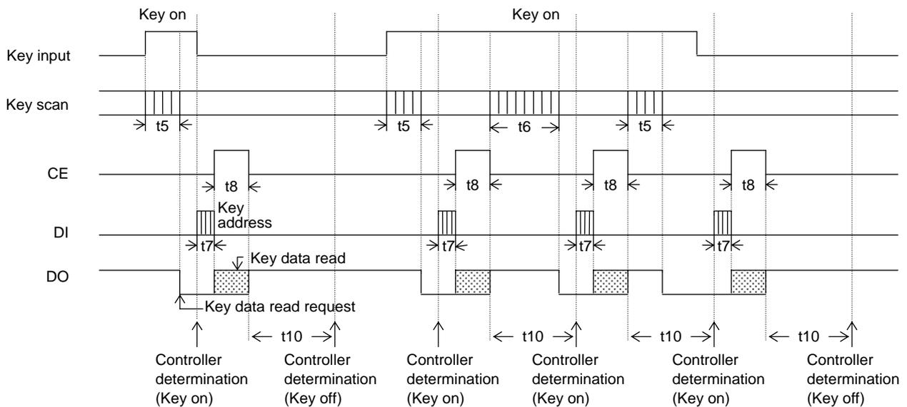
t5: Key scan execution time when the key data agreed for two key scans. (4800T(s))
