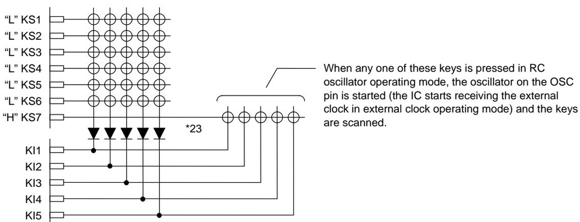
Note: \*23. These diodes are required to reliably recognize multiple key presses on the KS7 line when sleep mode state with only KS7 high, as in the above example.
