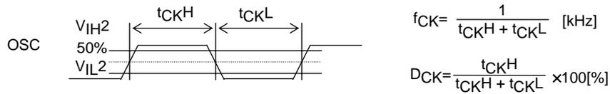
$$f_{CK} = \frac{1}{t_{CKH} + t_{CKL}} \text{ [kHz]}$$
