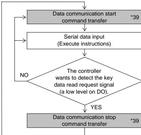
Note: \*39. In the case of the 4 line type CCB format, the transfers of data communication start command and data communication stop command are unnecessary, and, in the case of the 3 line type CCB format, these transfers are necessary.
