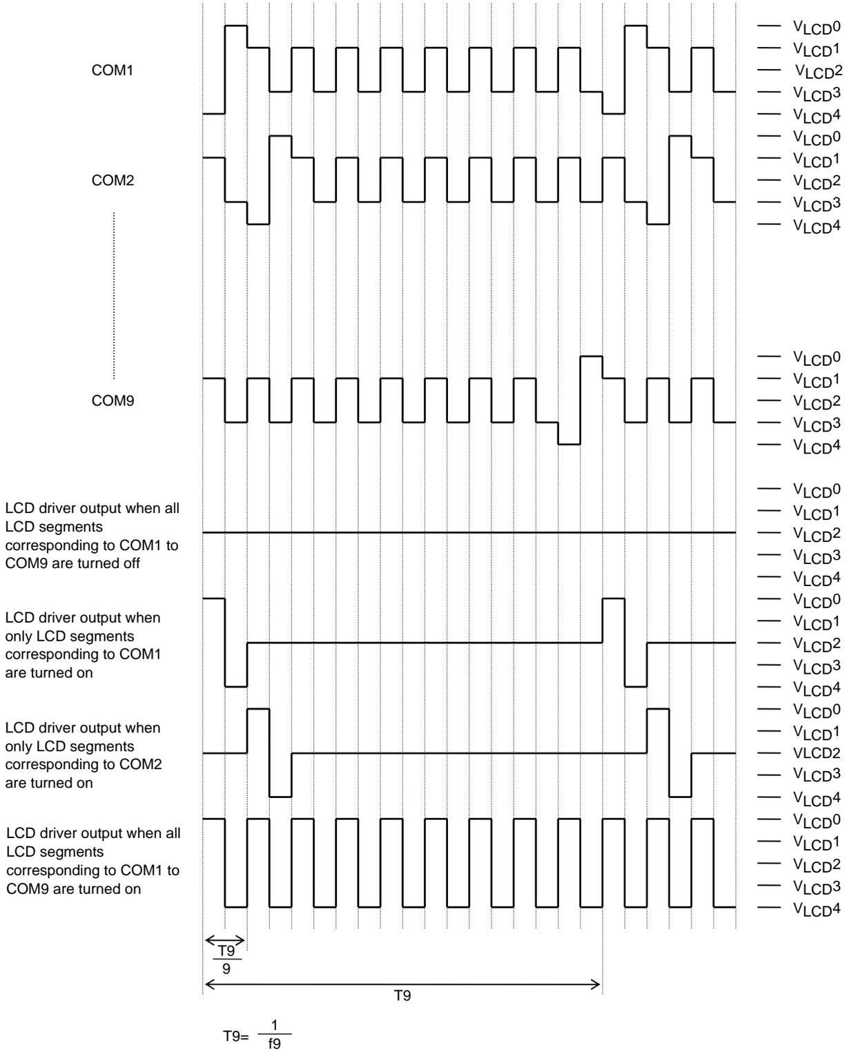
When a "set display technique" instruction with FC0 = 0, FC1 = 0 are executed:  $f_9 = \frac{f_{osc}}{3456}$  ,  $f_9 = \frac{f_{CK}}{3456}$
