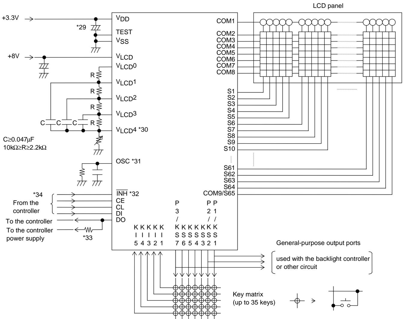
Note \*29. Add a capacitor to the logic block power supply line so that the logic block power supply voltage  $V_{DD}$  rise time when power is applied and the logic block power supply voltage  $V_{DD}$  fall time when power drops are both at least 1 ms, as the LC75812PT is reset by the  $V_{DET}$ .
