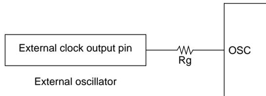
Note: \*28. Allowable current value at external clock output pin  $> \frac{V_{DD}}{R_g}$
