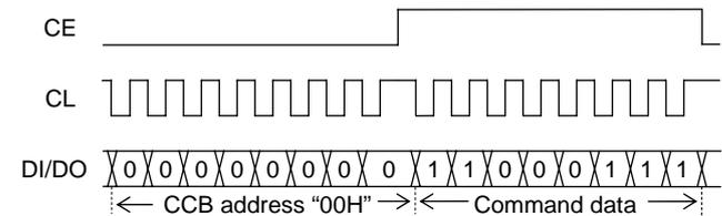
**Data Communication Flowchart of 4 Line Type or 3 Line Type CCB Format**
