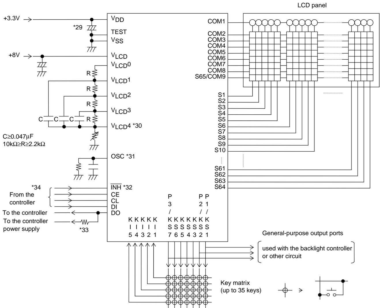
Note \*29. Add a capacitor to the logic block power supply line so that the logic block power supply voltage  $V_{DD}$  rise time when power is applied and the logic block power supply voltage  $V_{DD}$  fall time when power drops are both at least 1 ms, as the LC75812PT is reset by the  $V_{DET}$ .
