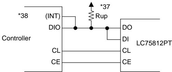
Note: \*37. Connect the pull-up resistor  $R_{up}$ . Select a resistance (between 1 to 10k $\Omega$ ) appropriate for the capacitance of the external wiring so that signal waveforms are not degraded.
