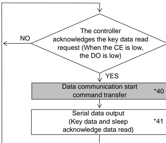
Note: \*40. In the case of the 4 line type CCB format, the transfer of data communication start command is unnecessary, and, in the case of the 3 line type CCB format, the transfer is necessary.
