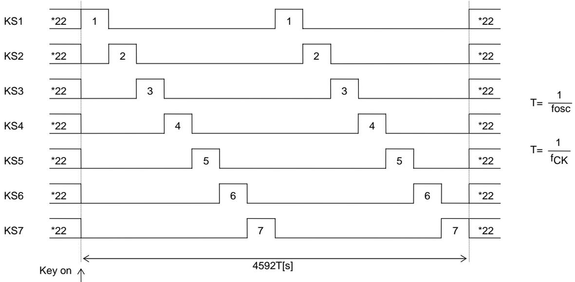
Note: \*22. Not that the high/low states of these pins are determined by the "set key scan output port/general-purpose output port state" instruction, and that key scan output signals are not output from pins that are set to low.
