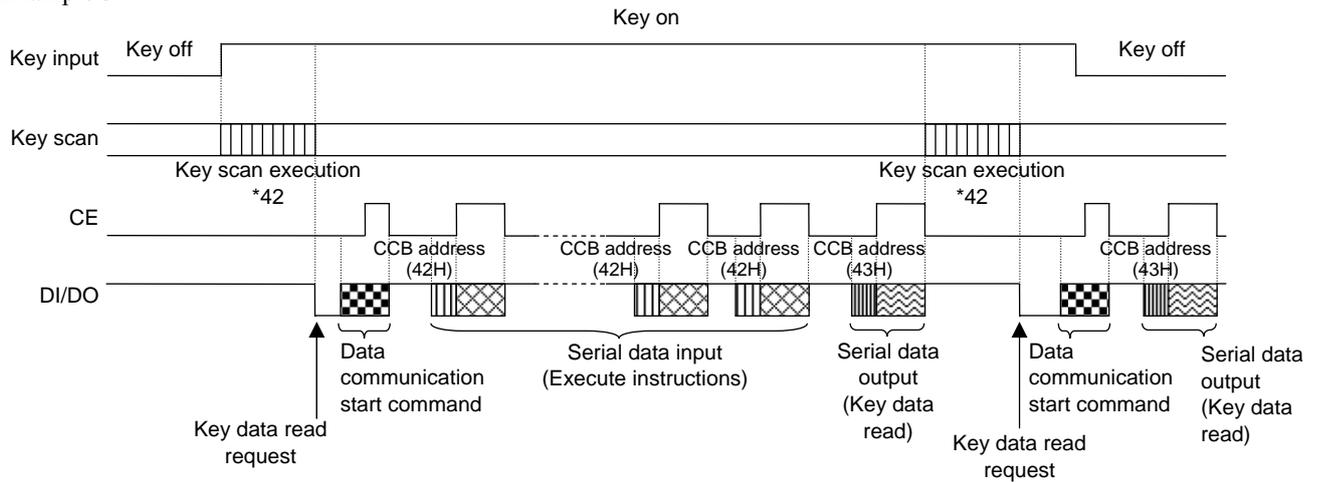
Note: \*42. When the key data agrees for two key scans, the key scan execution time is 4800T[s].
