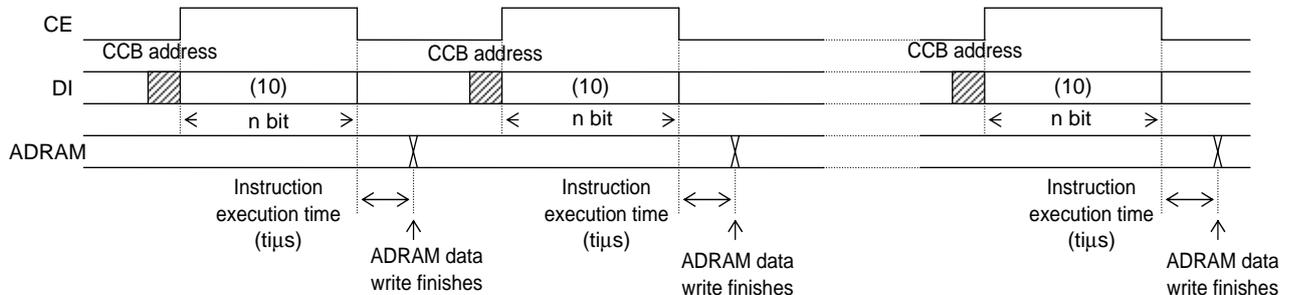
$$t_i = 13.5\mu\text{s} \times \left(\frac{n}{8} - 1\right)$$
