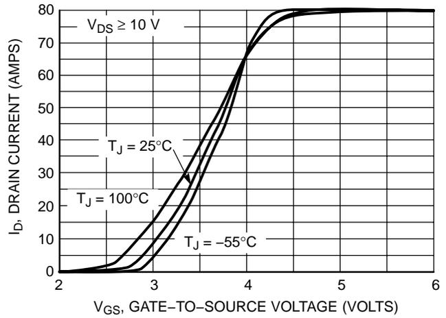
**Figure 2. Transfer Characteristics**
