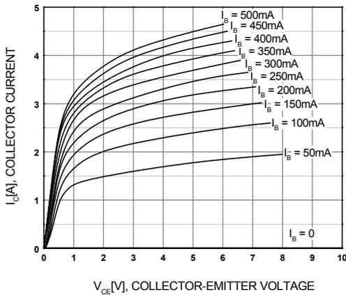
Figure 1. Static Characteristic
