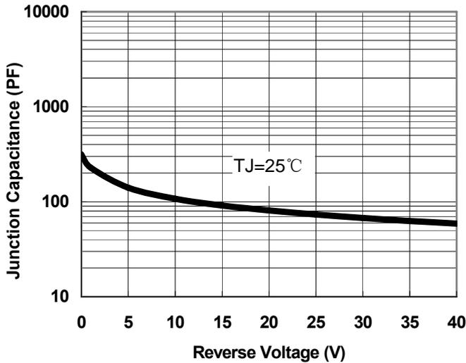
Fig.1-Typical Junction Capacitance
