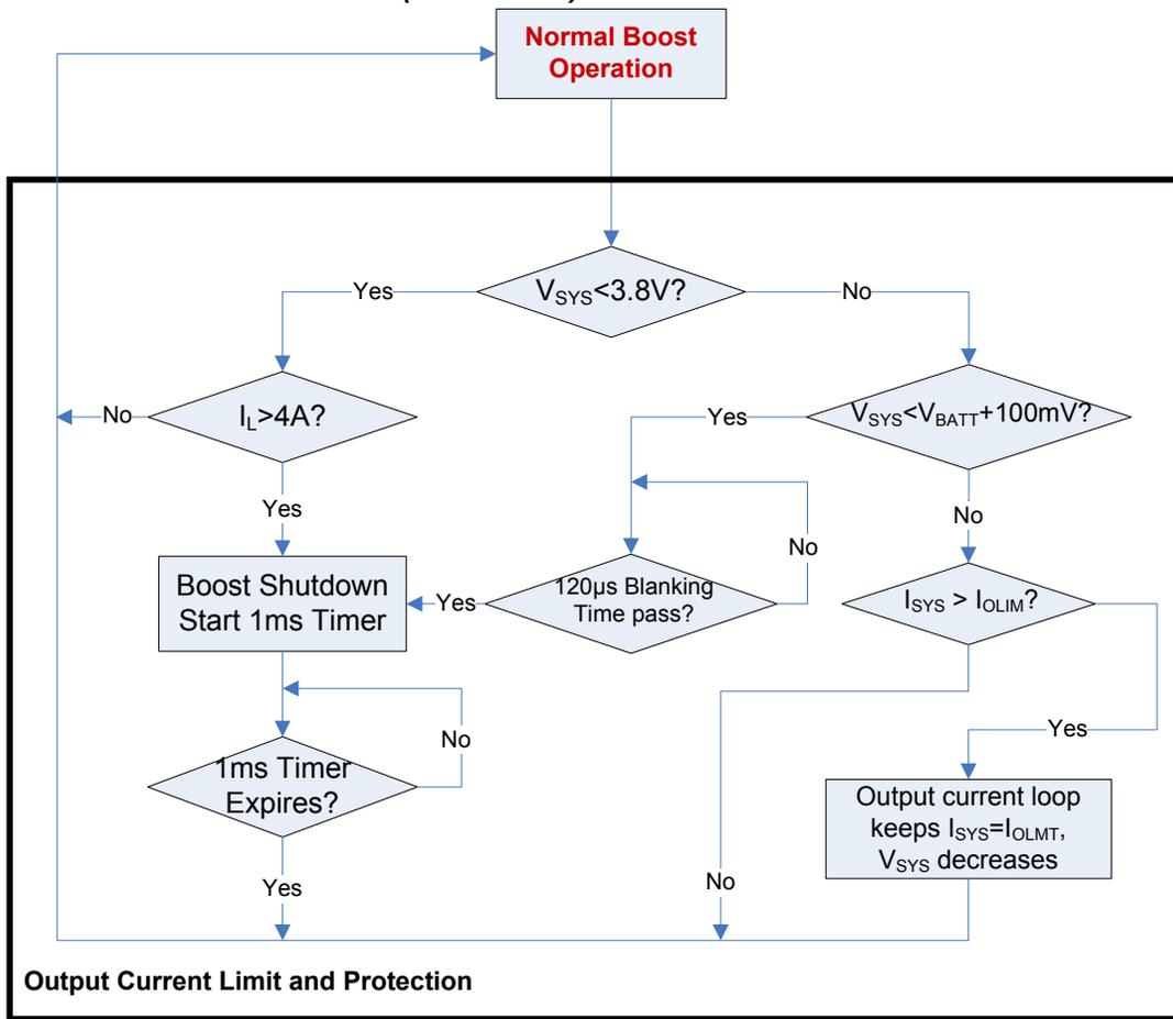
**Figure 6: Operation Flow Chart in Boost Mode**
