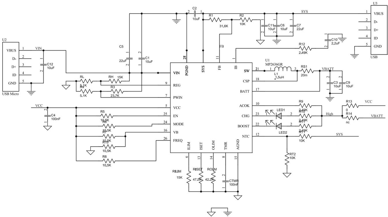
**Figure 14: The Detailed Application Circuit of MP2636**
