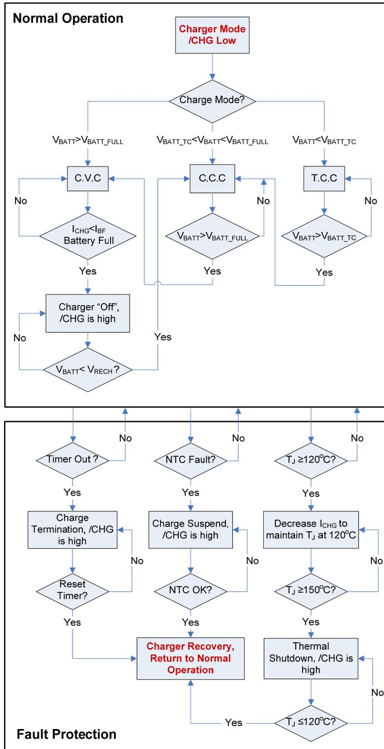
**Figure 4: Operation Flow Chart in Charger Mode**
