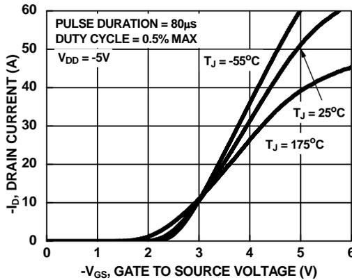
Figure 7. Transfer Characteristics
