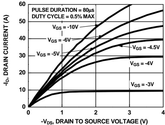
Figure 8. Saturation Characteristics
