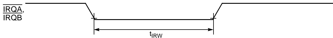
Figure 3-13 External Interrupt Timing (Negative-Edge-Sensitive)
