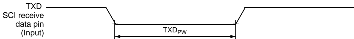
Figure 3-26 TXD Pulse Width
