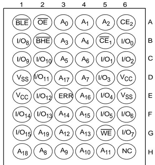
**Figure 6. 48-ball VFBGA (6 × 8 × 1.0 mm) Dual Chip Enable with ERR, Address MSB A19 at Ball H6**
