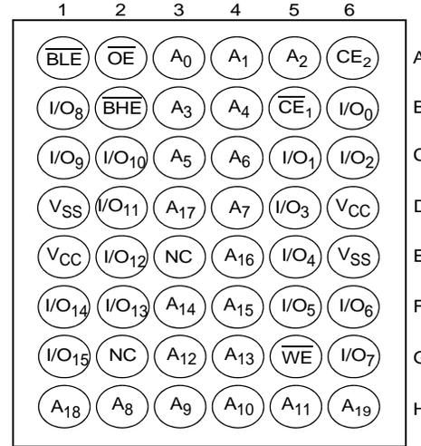
**Figure 3. 48-ball VFBGA (6 × 8 × 1.0 mm) Single Chip Enable without ERR, Address MSB A19 at Ball G2, CY7C1061G<sup>[3]</sup>**
