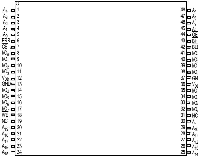
**Figure 8. 48-pin TSOP I (12 × 18.4 × 1 mm)**
