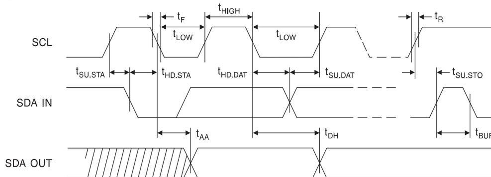
Figure 4-2. Write cycle timing SCL: Serial clock SDA: Serial data I/O
