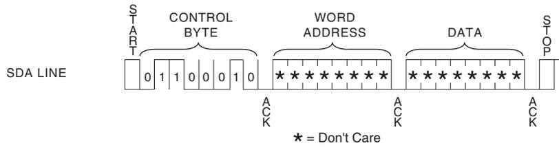
Figure 7-3. Clearing reversible write protect register (RSWP)
