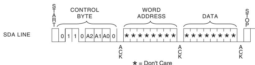
Figure 7-2. Setting reversible write protect register (RSWP)
