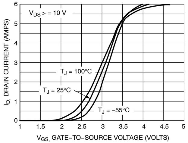
Figure 2. Transfer Characteristics
