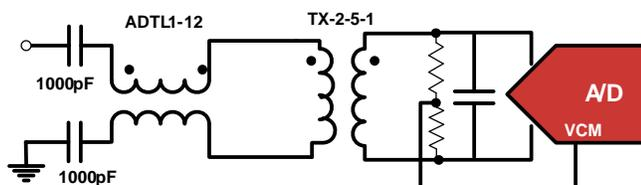
FIGURE 31. TRANSMISSION-LINE TRANSFORMER INPUT FOR HIGH IF APPLICATIONS
