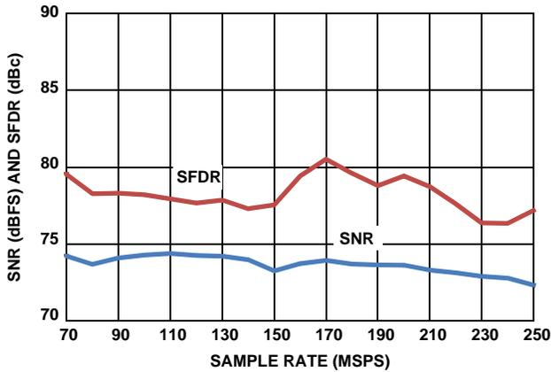
FIGURE 9. SNR AND SFDR vs f<sub>SAMPLE</sub>
