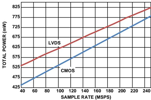
FIGURE 11. POWER vs f<sub>SAMPLE</sub> IN 3mA LVDS AND CMOS MODES
