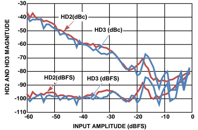
FIGURE 8. HD2 AND HD3 vs A<sub>IN</sub>
