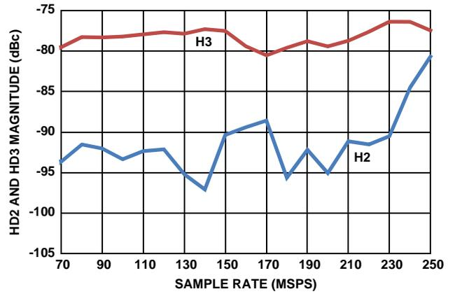
FIGURE 10. HD2 AND HD3 vs f<sub>SAMPLE</sub>
