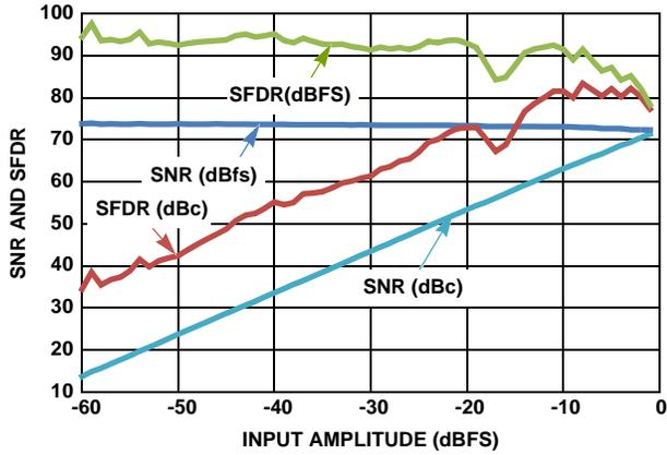
FIGURE 7. SNR AND SFDR vs A<sub>IN</sub>
