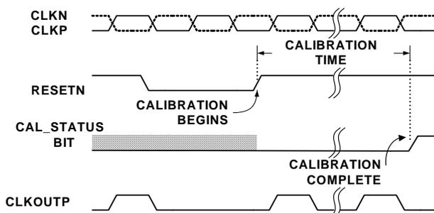
FIGURE 22. CALIBRATION TIMING
