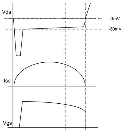
**Figure 4: Synchronous Rectification Operation at Light Load**
