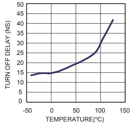
**Turn Off Delay (Load=10nF) vs. Temperature**
