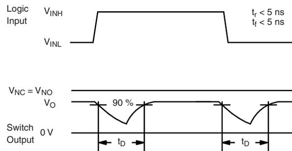
Figure 2. Break-Before-Make Interval
