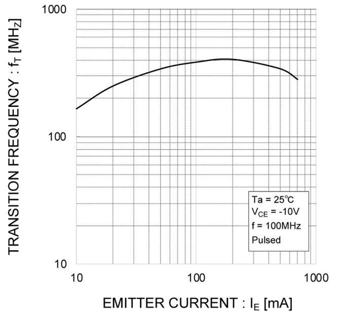
●Electrical characteristic curves( $T_a=25^\circ\text{C}$ ) <For Tr2(PNP)>
