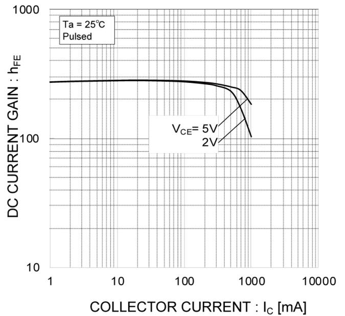
● Electrical characteristic curves ( $T_a=25^\circ\text{C}$ ) <For Tr1(NPN)>
