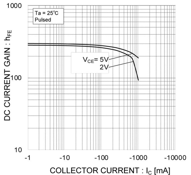
● Electrical characteristic curves ( $T_a = 25^\circ\text{C}$ ) <For Tr2(PNP)>
