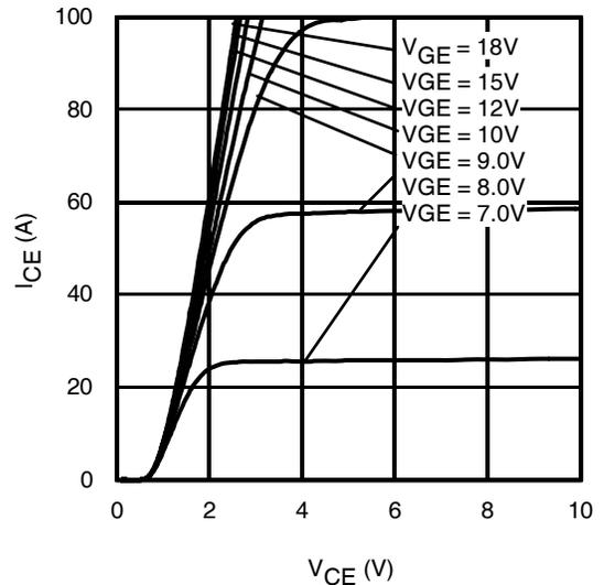
**Fig. 8** - Typ. IGBT Output Characteristics
