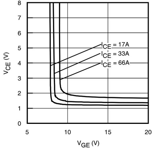
**Fig. 9** - Typical  $V_{CE}$  vs.  $V_{GE}$
