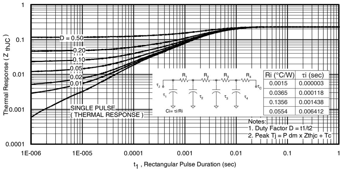
Fig 19. Maximum Transient Thermal Impedance, Junction-to-Case (IGBT)
