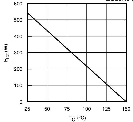
**Fig. 2** - Power Dissipation vs. Case Temperature
