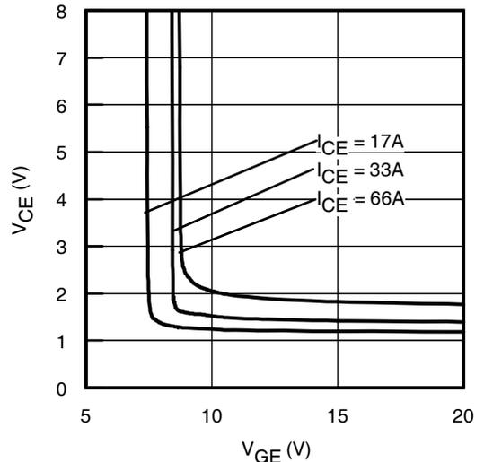
**Fig. 10** - Typical  $V_{CE}$  vs.  $V_{GE}$
