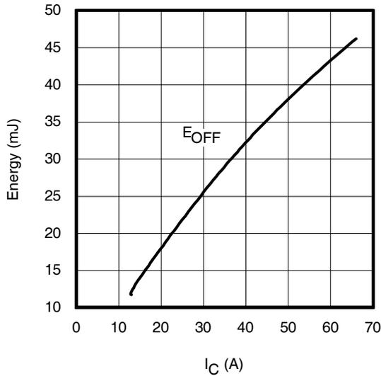
**Fig. 13 - Typ. Energy Loss vs.  $I_C$**
