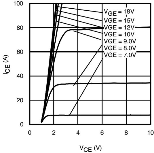
**Fig. 7** - Typ. IGBT Output Characteristics
