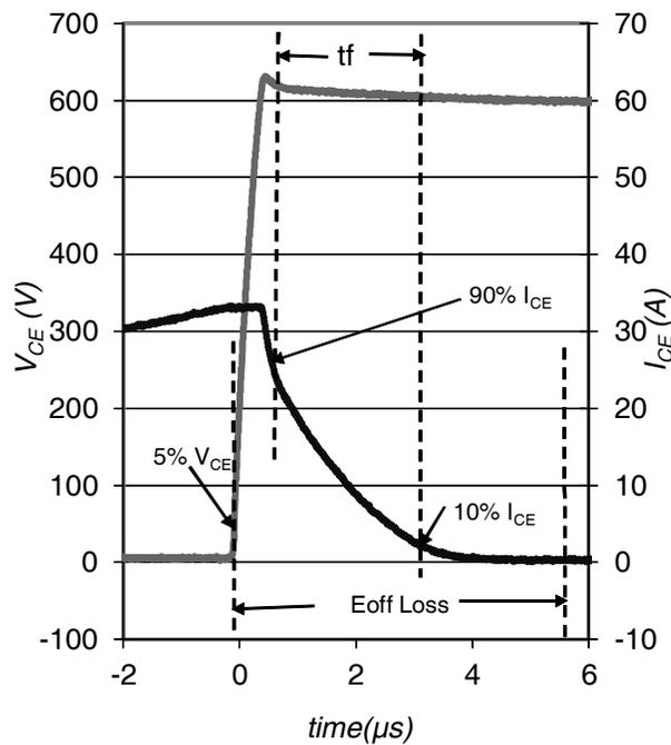
Fig. WF1 - Typ. Turn-off Loss Waveform
