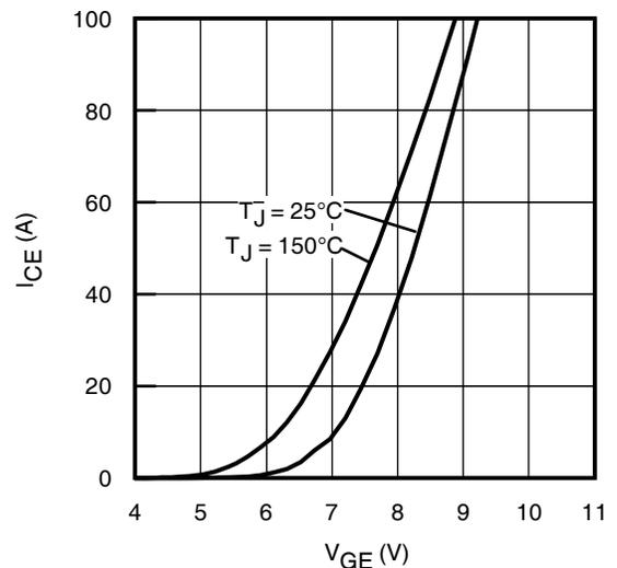
**Fig. 12** - Typ. Transfer Characteristics
