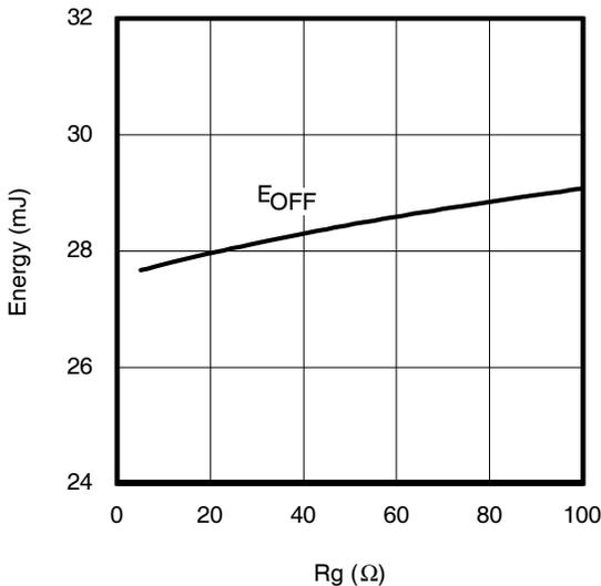
**Fig. 15 - Typ. Energy Loss vs.  $R_G$**
