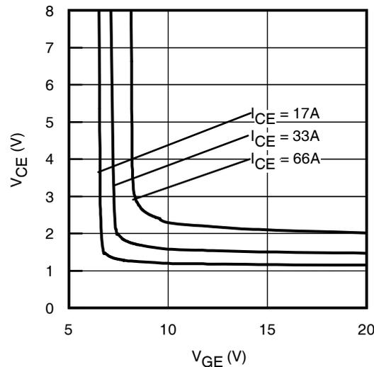
**Fig. 11** - Typical  $V_{CE}$  vs.  $V_{GE}$
