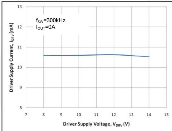
Figure 14. Driver Supply Current vs. Driver Supply Voltage
