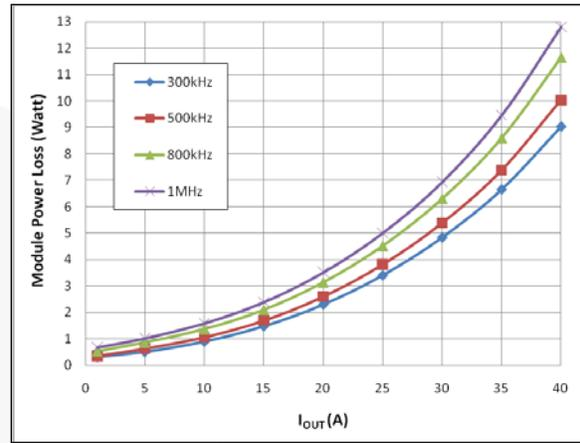
Figure 7. Module Power Loss vs. Output Current
