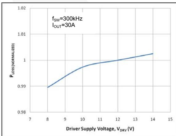
Figure 10. Power Loss vs. Driver Supply Voltage
