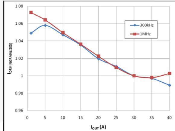
Figure 15. Driver Supply Current vs. Output Current
