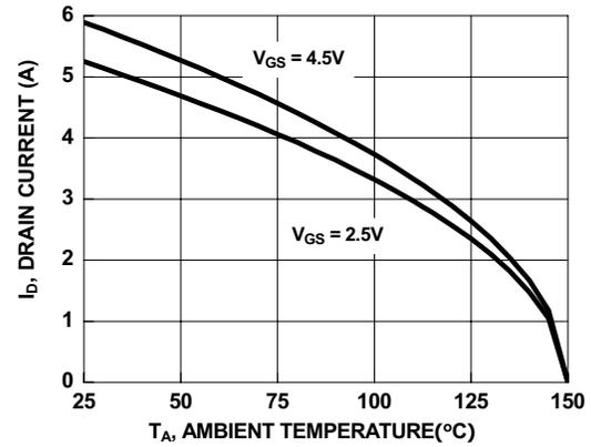
Figure 10. Maximum Continuous Drain Current vs Ambient Temperature
