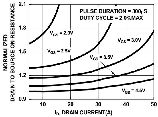
Figure 2. On-Resistance vs Drain Current and Gate Voltage
