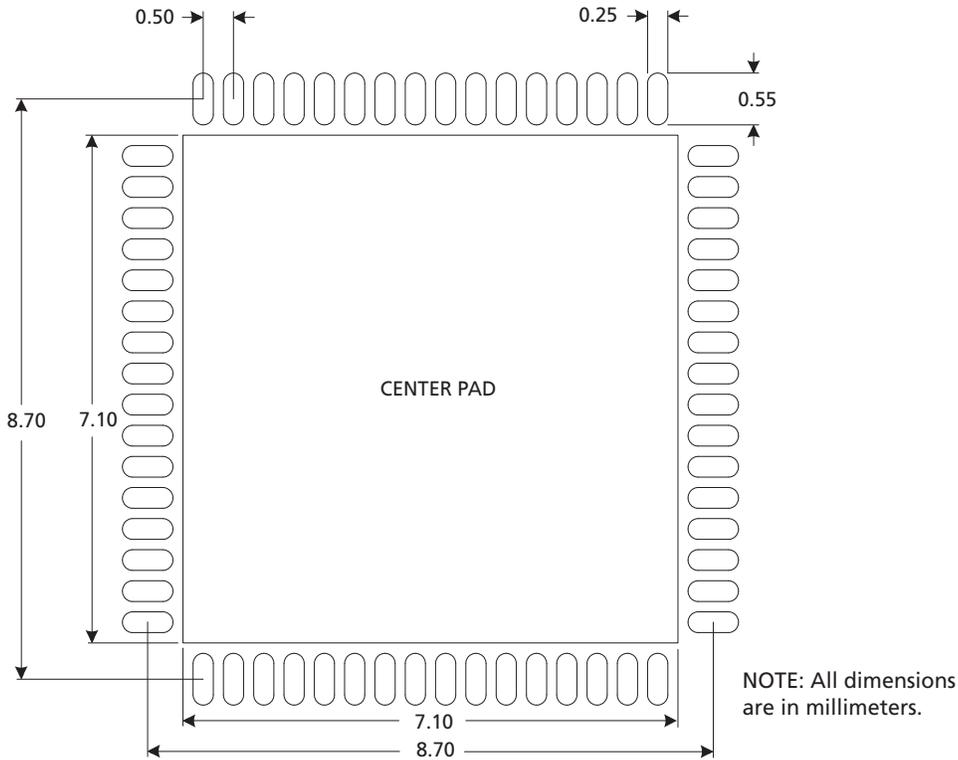
The center pad of the PCB footprint should be connected to the ground plane by a minimum of 36 vias.
