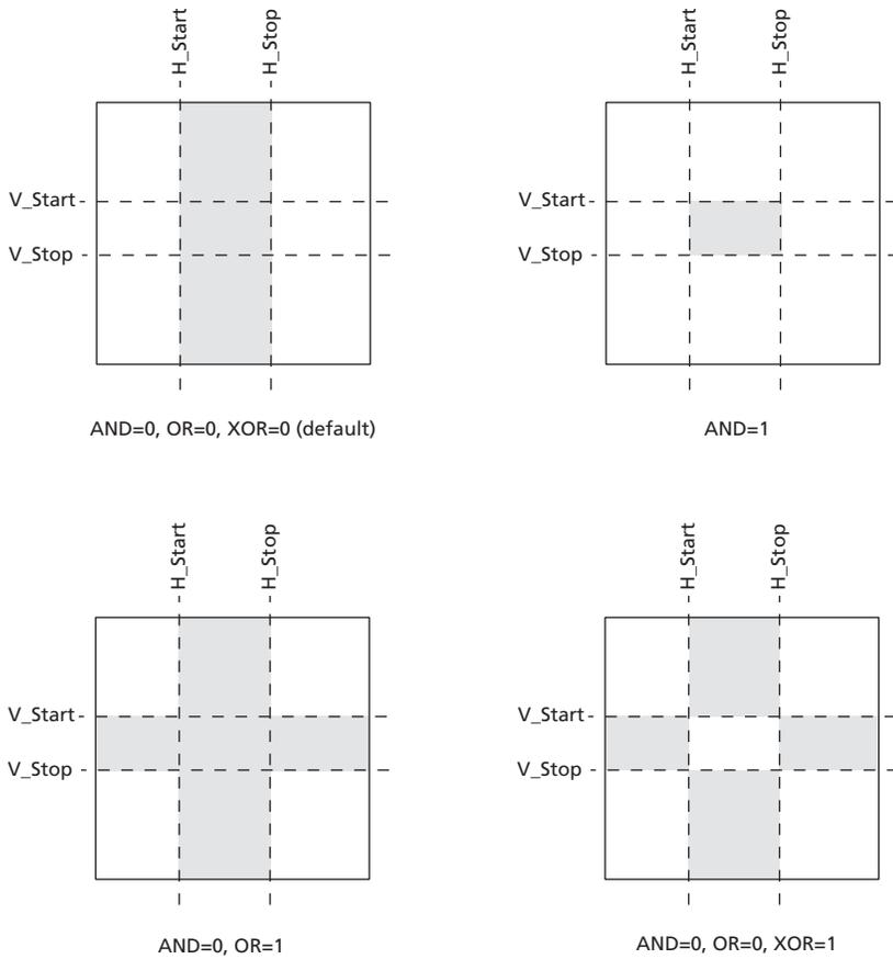
Shading indicates when USER\_x signal is active
