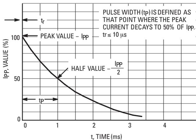
Figure 5. Pulse Waveform
