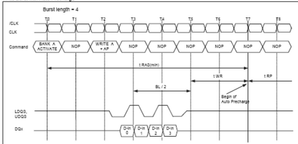
Note:  $t_{WR}$  starts at the first rising edge of clock after the last valid edge of the 4 DQSx.
