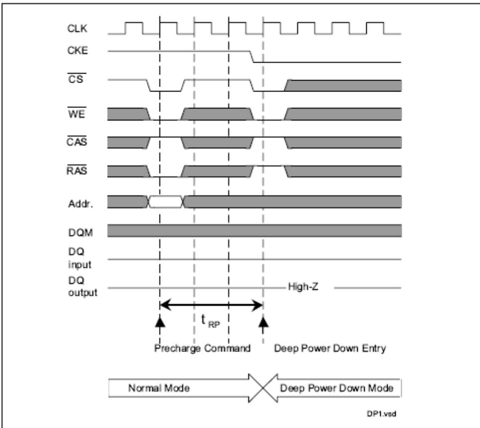
The deep power down mode has to be maintained for a minimum of 100 $\mu$ s.
