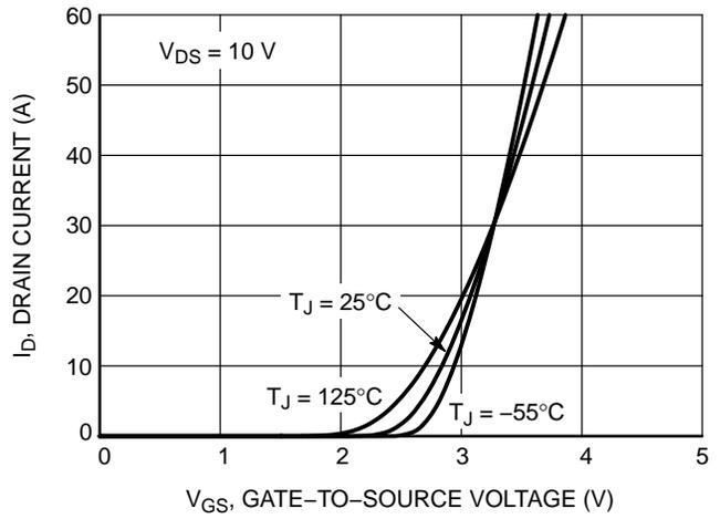
Figure 2. Transfer Characteristics
