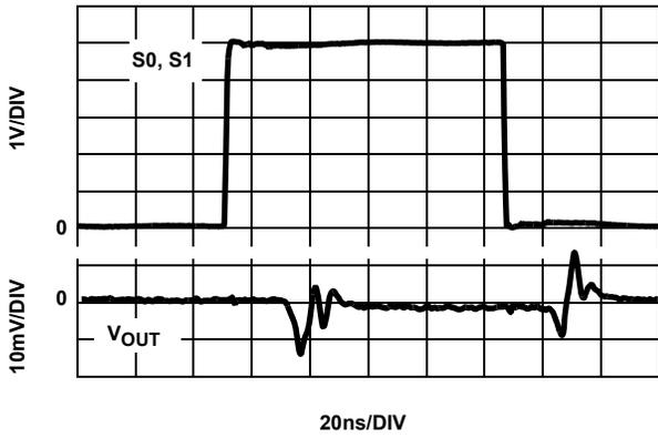
FIGURE 13. CHANNEL TO CHANNEL SWITCHING GLITCH
