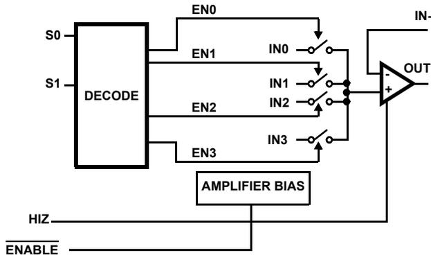
ENABLE pin must be low in order to activate the HIZ state
