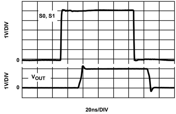
FIGURE 14. CHANNEL TO CHANNEL TRANSIENT RESPONSE
