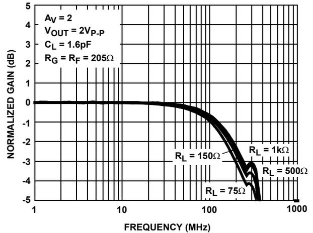
FIGURE 4. LARGE SIGNAL GAIN vs FREQUENCY vs  $R_L$
