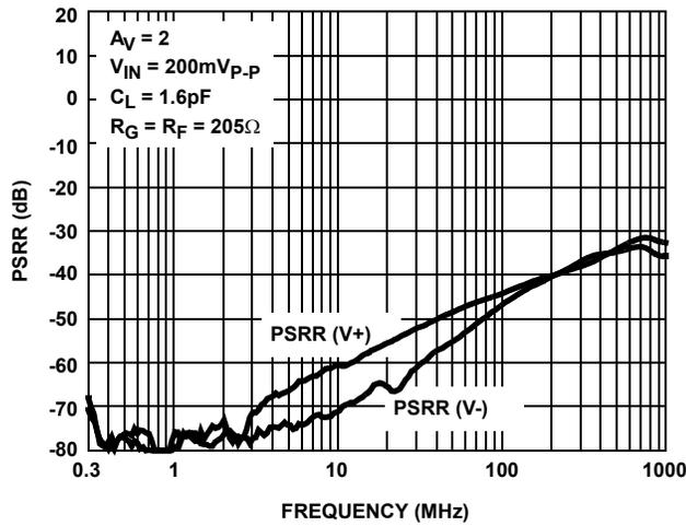
FIGURE 9. PSRR CHANNELS
