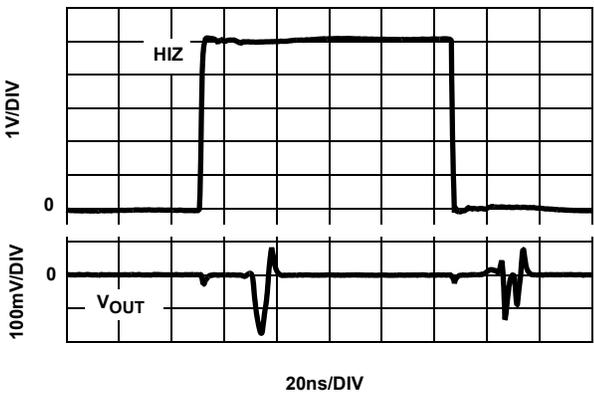
FIGURE 17. HIZ SWITCHING GLITCH  $V_{IN} = 0V$ ,  $A_V = 2$
