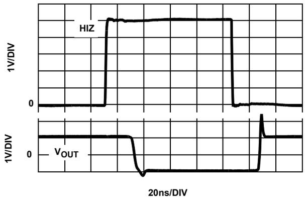
FIGURE 18. HIZ TRANSIENT RESPONSE  $V_{IN} = 1V$ ,  $A_V = 2$
