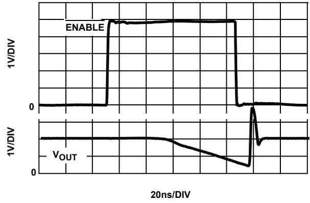
FIGURE 16. ENABLE TRANSIENT RESPONSE  $V_{IN} = 1V$ ,  $A_V = 2$
