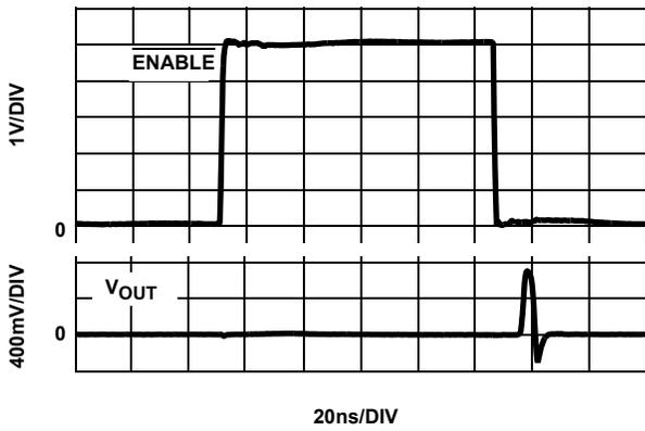
FIGURE 15. ENABLE SWITCHING GLITCH  $V_{IN} = 0V$ ,  $A_V = 2$
