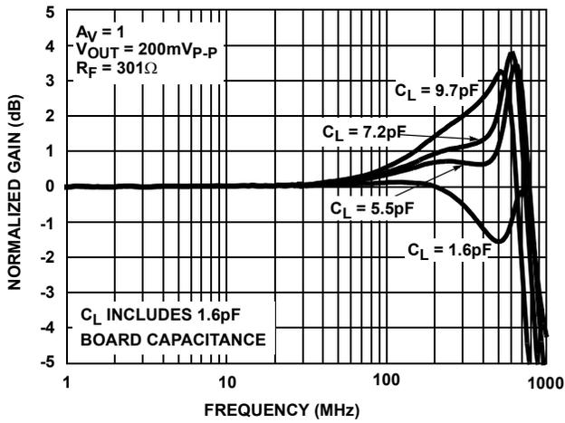
FIGURE 1. SMALL SIGNAL GAIN vs FREQUENCY vs  $C_L$
