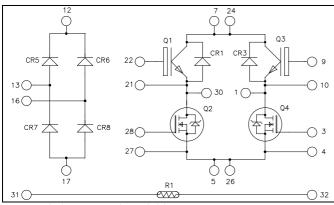
Top switches: Trench + Field Stop IGBT3
