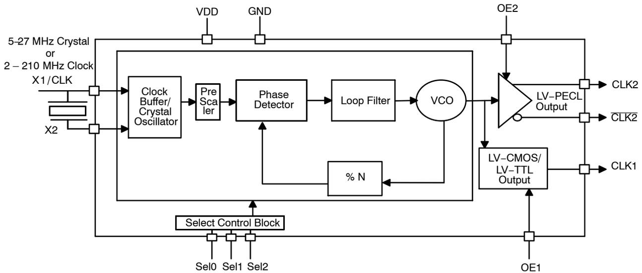
**Figure 1. NB3N3020 Simplified Logic Diagram**
